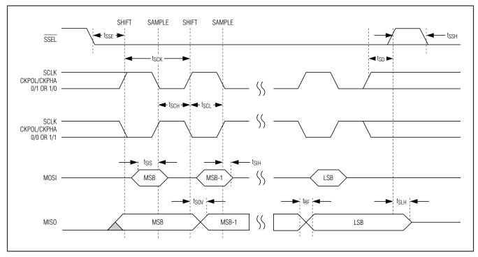
Figure 2. SPI Slave Timing
