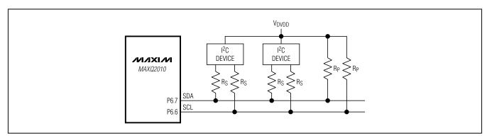
Figure 3. Series Resistors (R<sub>S</sub>) for Protecting Against High-Voltage Spikes
