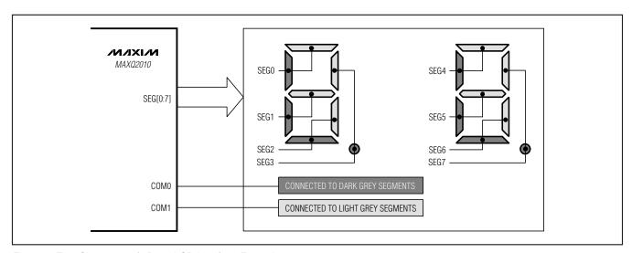
Figure 8. Two-Character, 1/2 Duty, LCD Interface Example
