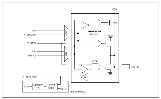
Figure 6. Type C/D Port Pin Schematic
