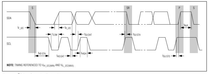
Figure 4. I<sup>2</sup>C Bus Controller Timing Diagram
