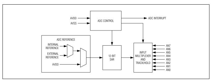
Figure 7. ADC Block Diagram
