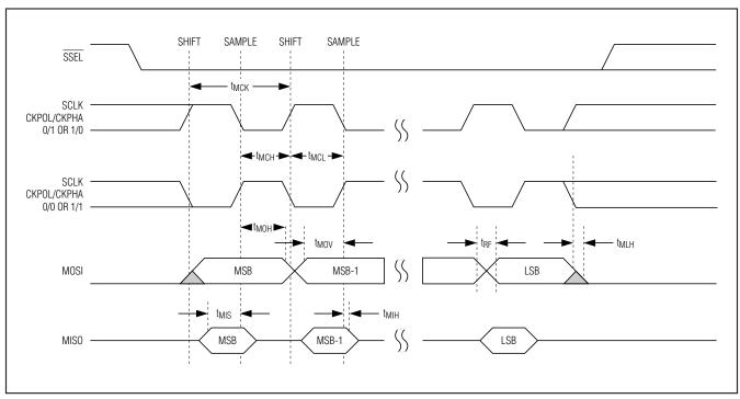
Figure 1. SPI Master Timing
