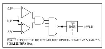
Figure 3b. INVALID Functional Diagram, INVALID High
