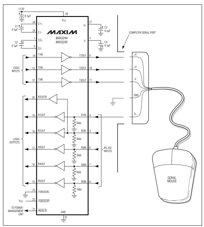
Figure 11b. Mouse Driver Test Circuit
