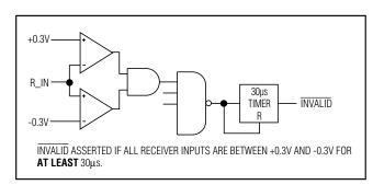
Figure 3a. INVALID Functional Diagram, INVALID Low
