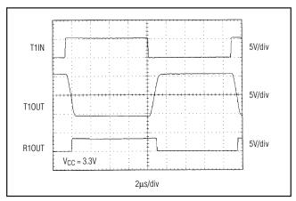
Figure 8. MAX3224/MAX3226/MAX3244 Loopback Test Result at 120kbps
