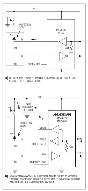
Figure 2. The MAX3244/MAX3245 detect RS-232 activity when the UART and interface are shut down.
