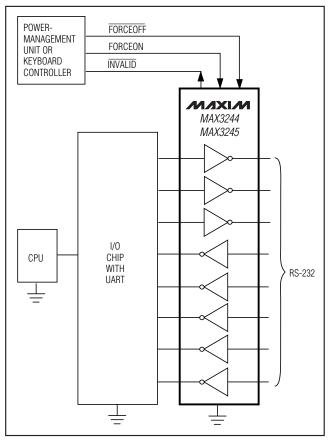
Figure 1. Interface Under Control of PMU
