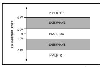
Figure 4a. Receiver Positive/Negative Thresholds for INVALID
