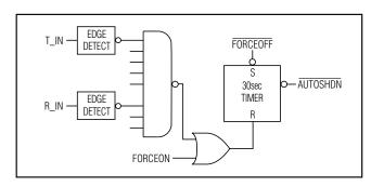
Figure 3c. AutoShutdown Plus Logic
