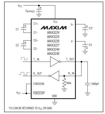
Figure 7. Loopback Test Circuit
