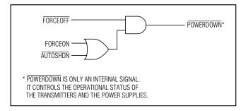
Figure 3d. Power-Down Logic
