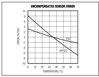
Figure 6. Sensor Characteristics Before Compensation
