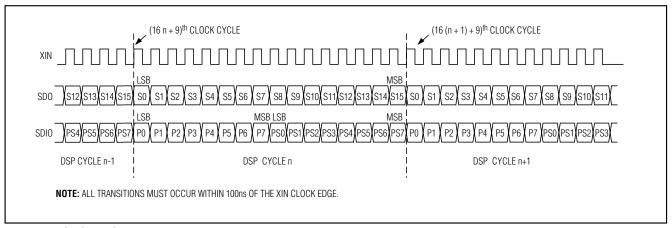
Figure 4. DSP Serial Output Timing Diagram
