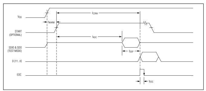
Figure 5. MAX1462 Conversion Timing
