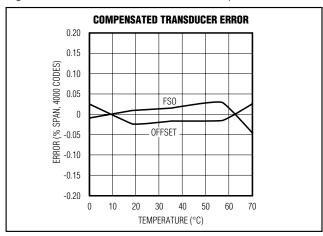
Figure 7. Compensated Sensor/MAX1462 Pair
