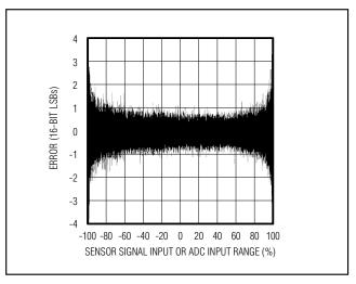
Figure 2b. Analog Front-End Differential Nonlinearity (DNL) (typ)
