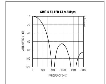
Figure 2. Sinc 5 Filter Frequency Response
