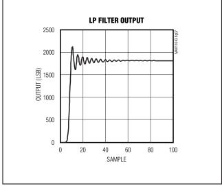
Figure 7. LP Filter Response to a Step Input
