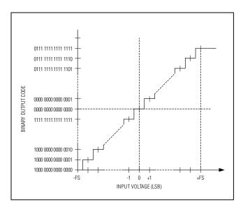
Figure 3. Two's Complement Transfer Function
