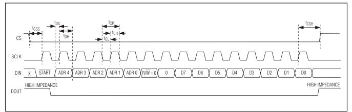
Figure 9. SPI 8-Bit Write Operation
