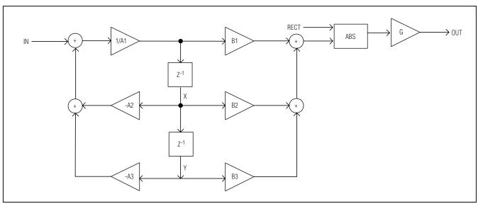
Figure 4. Single Programmable 2nd-Order Filter Section
