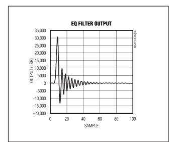
Figure 6. EQ Filter Response to a Step Input
