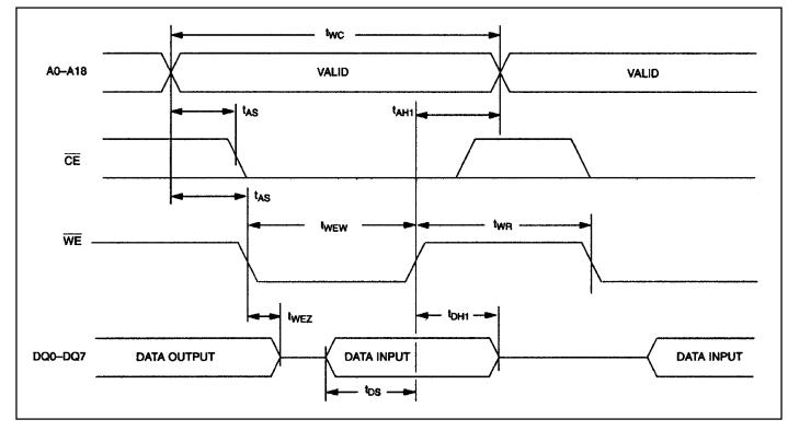
Figure 6. Write Cycle Timing, Write-Enable Controlled
