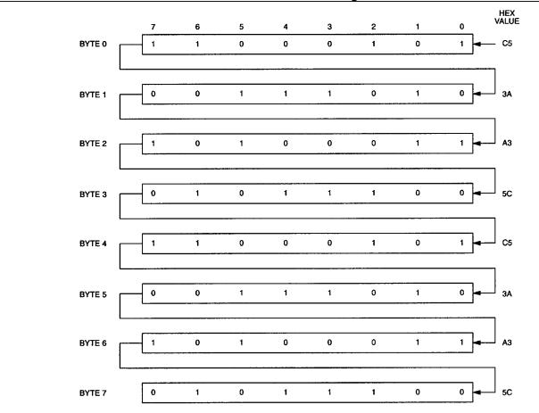
**NOTE**: THE PATTERN RECOGNITION IN HEX IS C5, 3A, A3, 5C, C5, 3A, A3, 5C. THE ODDS OF THIS PATTERN BEING ACCIDENTALLY DUPLICATED AND CAUSING INADVERTENT ENTRY TO THE PHANTOM CLOCK IS LESS THAN 1 IN  $10^{19}$ . THIS PATTERN IS SENT TO THE PHANTOM CLOCK LSB TO MSB.
