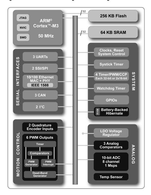
Figure 1-1. Stellaris® 8000 Series High-Level Block Diagram
