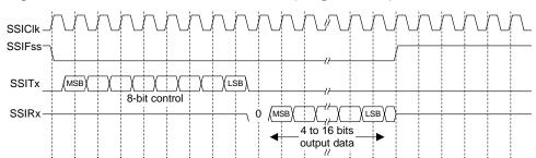
Figure 12-10. MICROWIRE Frame Format (Single Frame)
