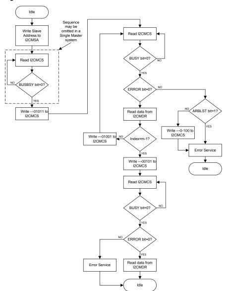
Figure 13-10. Master Burst RECEIVE
