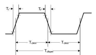
Figure 19-3. External XTLP Oscillator Characteristics
