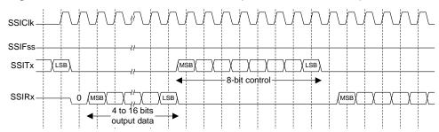
Figure 12-11. MICROWIRE Frame Format (Continuous Transfer)
