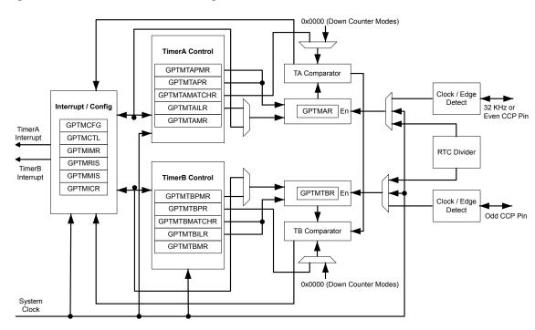
Figure 9-1. GPTM Module Block Diagram
