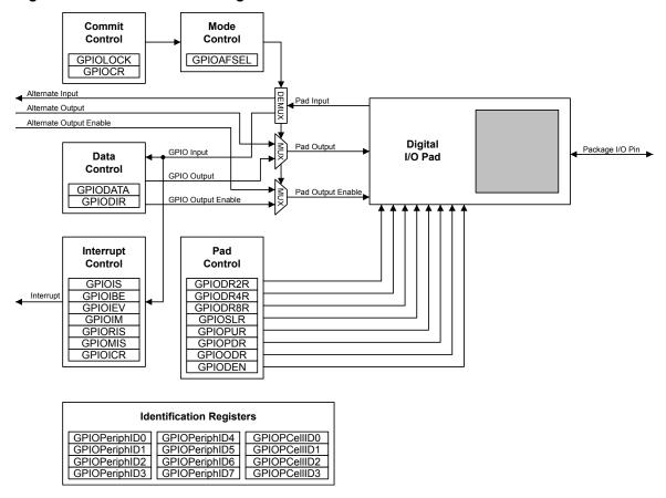
Figure 8-1. GPIO Port Block Diagram
