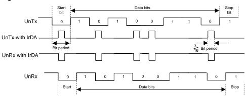
Figure 11-3. IrDA Data Modulation
