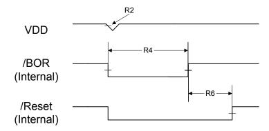
Figure 19-13. Software Reset Timing
