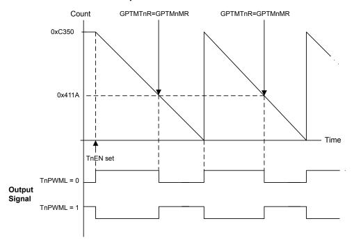
Figure 9-4. 16-Bit PWM Mode Example
