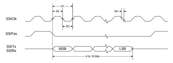
Figure 19-5. SSI Timing for MICROWIRE Frame Format (FRF=10), Single Transfer
