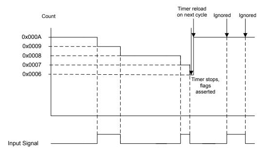
Figure 9-2. 16-Bit Input Edge Count Mode Example
