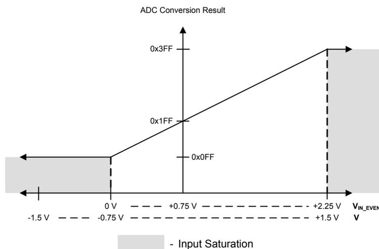
Figure 11-4. Differential Sampling Range,  $V_{IN\_ODD} = 2.25\text{ V}$
