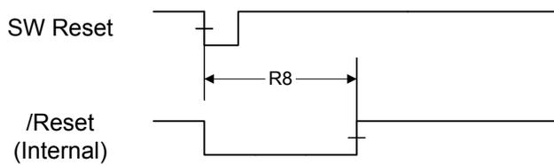
**Figure 19-13. Watchdog Reset Timing**
