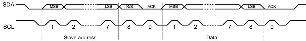
The first seven bits of the first byte make up the slave address (see Figure 14-5 on page 334). The eighth bit determines the direction of the message. A zero in the R/S position of the first byte means that the master will write (send) data to the selected slave, and a one in this position means that the master will receive data from the slave.
