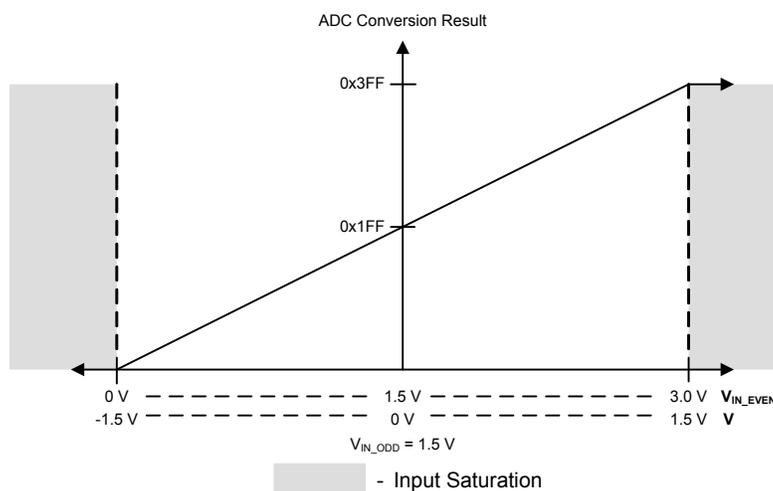
**Figure 11-3. Differential Sampling Range,  $V_{IN\_ODD} = 0.75$  V**
