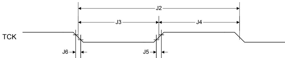
Figure 20-7. JTAG Test Access Port (TAP) Timing
