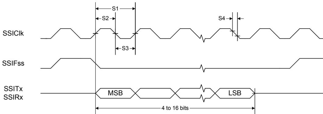
Figure 20-4. SSI Timing for MICROWIRE Frame Format (FRF=10), Single Transfer
