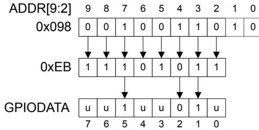
During a read, if the address bit associated with the data bit is set to 1, the value is read. If the address bit associated with the data bit is set to 0, it is read as a zero, regardless of its actual value. For example, reading address GPIODATA + 0x0C4 yields as shown in Figure 8-3 on page 142.
