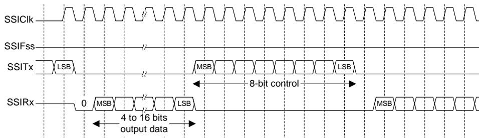
In the MICROWIRE mode, the SSI slave samples the first bit of receive data on the rising edge of SSIClk after SSIFss has gone Low. Masters that drive a free-running SSIClk must ensure that the SSIFss signal has sufficient setup and hold margins with respect to the rising edge of SSIClk.
