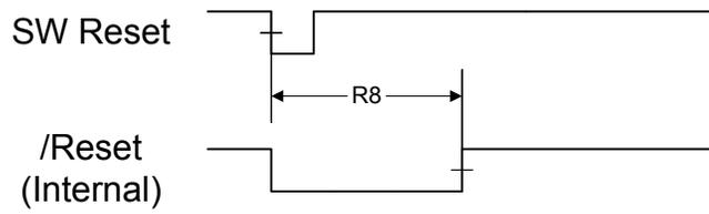
**Figure 20-13. Watchdog Reset Timing**
