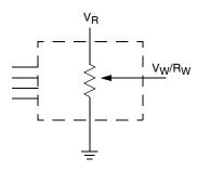
Three terminal Potentiometer; Variable voltage divider
