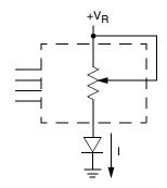
Two terminal Variable Resistor; Variable current
