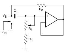
$$\begin{split} Z_{IN} = R_2 + s \; R_2 \; (R_1 + R_3) \; C_1 = R_2 + s \; \text{Leq} \\ (R_1 + R_3) >> R_2 \end{split}$$
