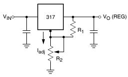
$V_{O}(REG) = 1.25V (1+R_2/R_1)+I_{adj} R_2$
