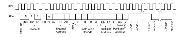
Figure 6. Increment/Decrement Timing Limits
