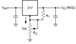
$V_O (REG) = 1.25V (1+R_2/R_1)+I_{adj} R_2$
