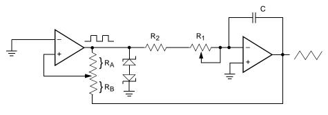
$\begin{array}{l} \mbox{frequency} \propto R_1,\,R_2,\,C \\ \mbox{amplitude} \propto R_A,\,R_B \end{array}$
