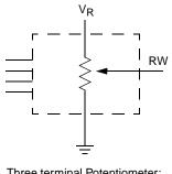
Three terminal Potentiometer; Variable voltage divider
