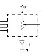
Two terminal Variable Resistor; Variable current
