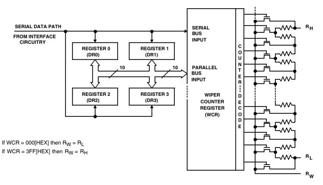
FIGURE 1. DETAILED POTENTIOMETER BLOCK DIAGRAM
