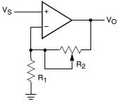
$V_0 = (1 + R_2/R_1)V_S$
