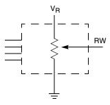
Three terminal Potentiometer; Variable voltage divider
