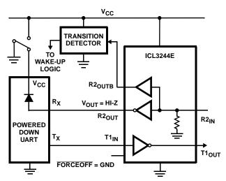
FIGURE 3. DISABLED RECEIVERS PREVENT POWER DRAIN
