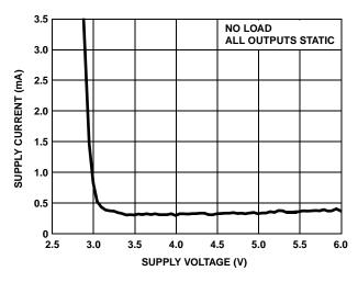
FIGURE 20. SUPPLY CURRENT vs SUPPLY VOLTAGE
