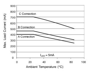
Figure 1. Current Derating Curve
