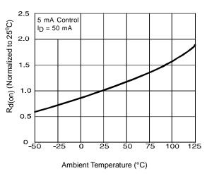
Figure 2. Typical Normalized On-Resistance
