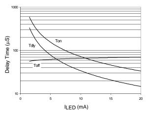
Figure 7.Typical Delay Times
