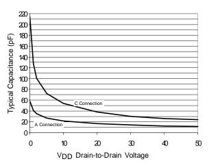
Figure 9. Typical Output Capacitance
