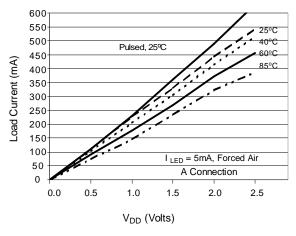
Figure 3. Typical On-Characteristic A Connection
