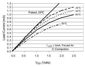
Figure 4. Typical On-Characteristic C Connection
