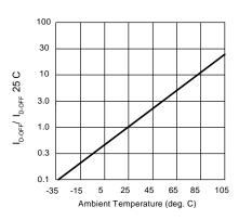
Figure 5. Typical Normalized Off-State Leakage
