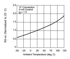
Figure 4. Typical Normalized On-Resistance
