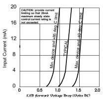
Figure 6. Input Characteristics (Current Controlled)
