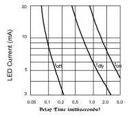
Figure 7. Typical Delay Times
