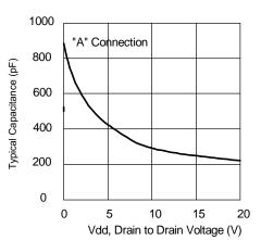
Figure 2. Typical Output Capacitance
