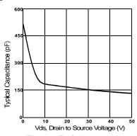
Figure 9. Typical Output Capacitance
