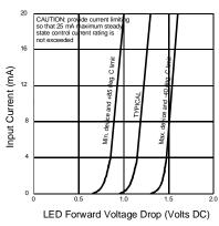
Figure 6. Input Characteristics (Current Controlled)
