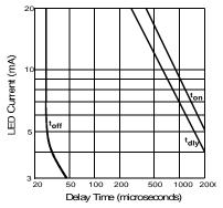
Figure 7. Typical Delay Times
