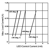
Figure 2. Typical Control Current Requirements
