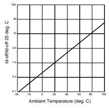
Figure 5. Typical Normalized Off-State Leakage
