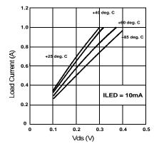
Figure 3. Typical On-Characteristics
