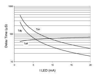
Figure 7.Typical Delay Times
