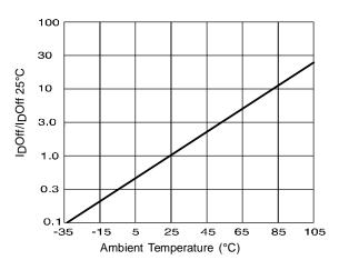
Figure 5. Typical Normalized Off-State Leakage
