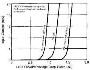
Figure 6. Input Characteristics (Current Controlled)
