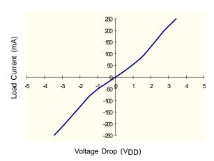
Figure 3.Typical On Characteristics
