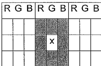
2 dots defect included defect dot "X" is defined as follows.
