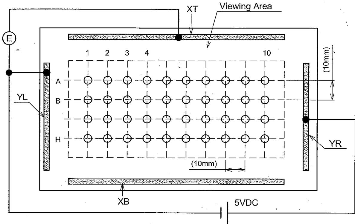
(b) Y axis linearity testing method , VXT-VXB=5V , VOUT=VYR.
