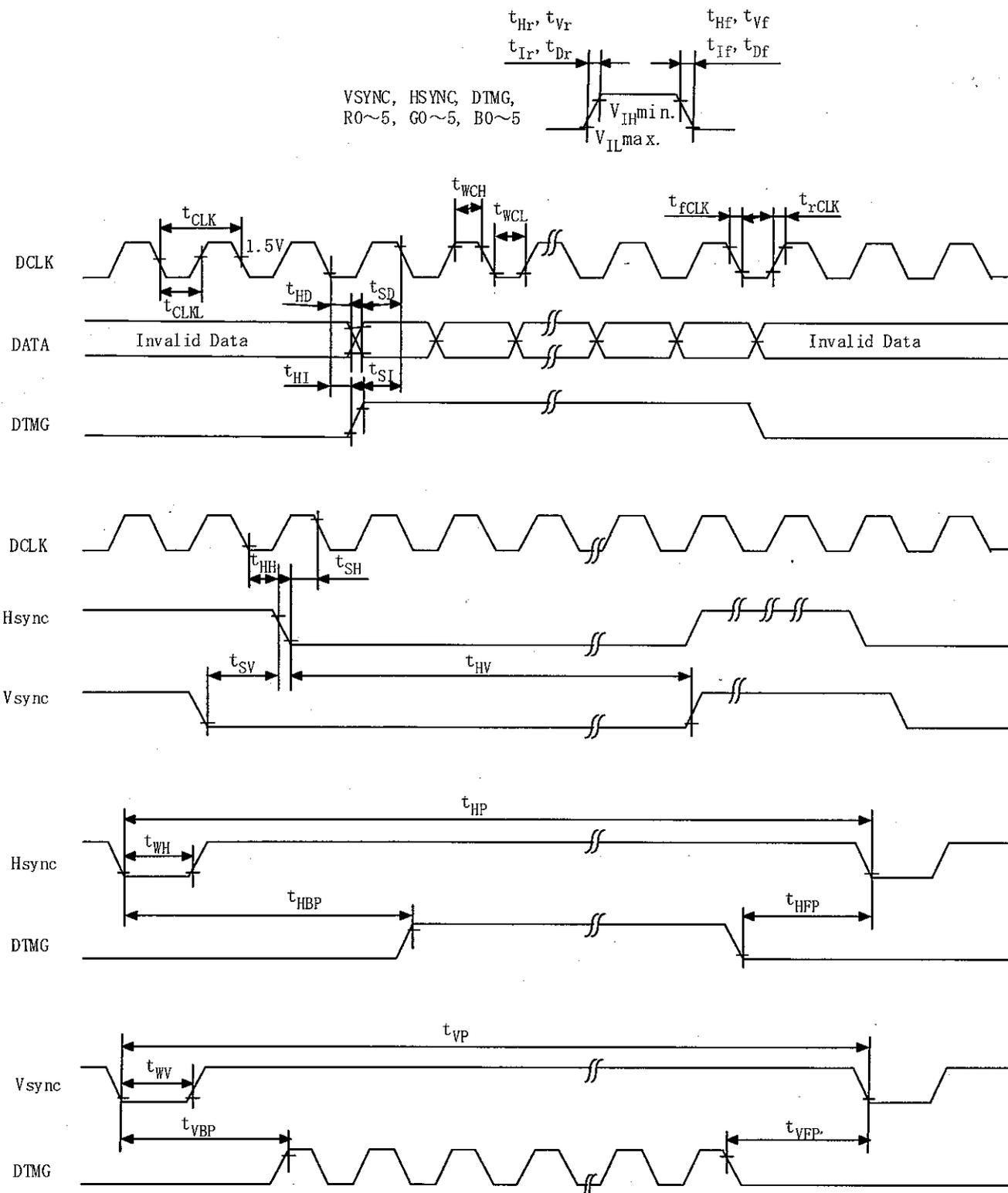
Note 1 : DTMG is definition of the above timing for Hsync and Vsync.
