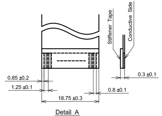
Note 1 : Measurement when adding  $9.8 \times 10^4$  Pa at the measuring point.
