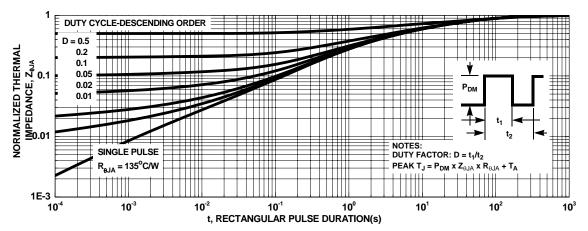
Figure 14. Transient Thermal Response Curve
