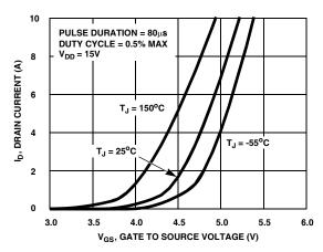
Figure 4. Transfer Characteristics
