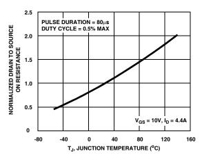
Figure 2. Normalized On-Resistance vs Junction Temperature
