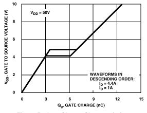
Figure 5. Gate Charge Characteristics
