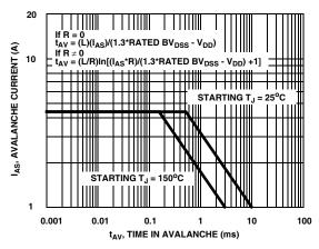
Figure 8. Uncalamped Inductive Switching Capability
