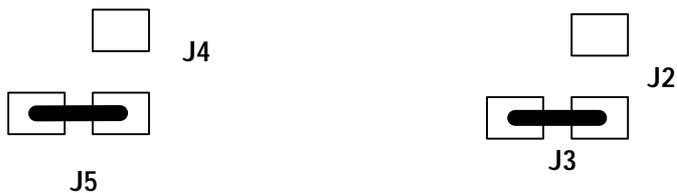
6-2-4. The metal-bezel is on ground as following.
