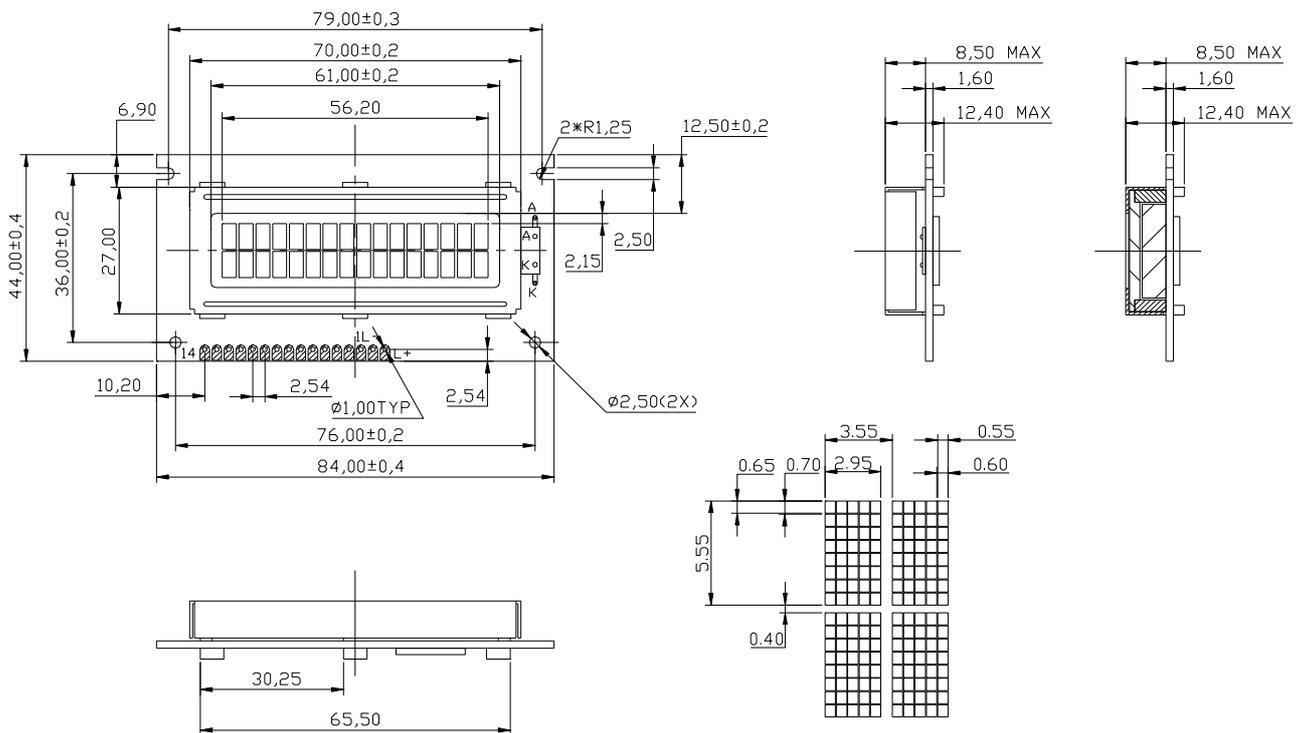
Figure 2.0 External Dimensions For DEM 16217 SYH-LY
