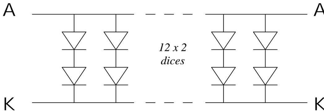
Figure 5.0 Backlight for DEM 16217 SYH-LY
