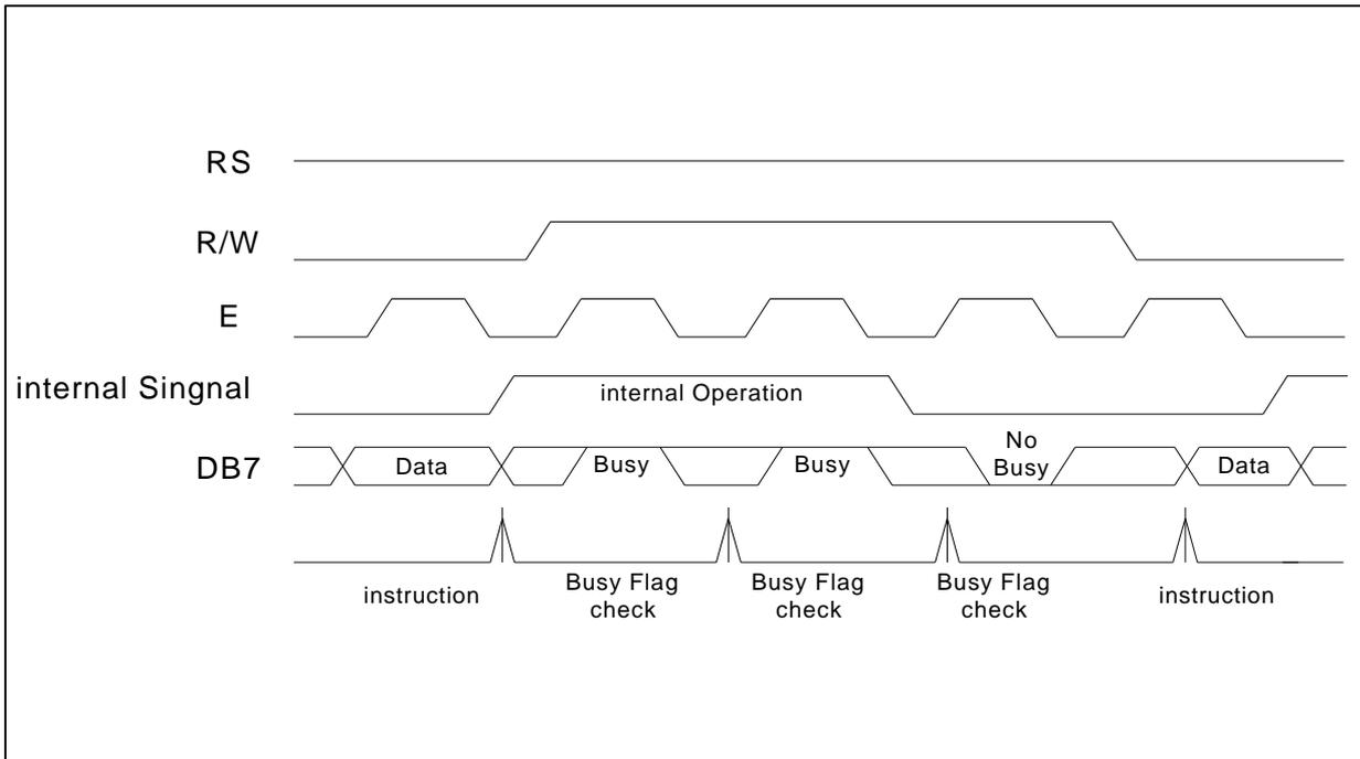
Figure 6.0 Example of 8-bit bus mode timing diagram
