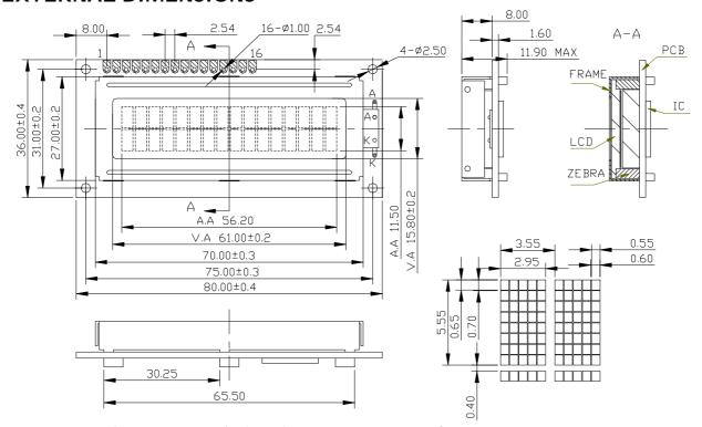
Figure 2.0 External Dimensions For DEM 16216 FGH-LA-N
