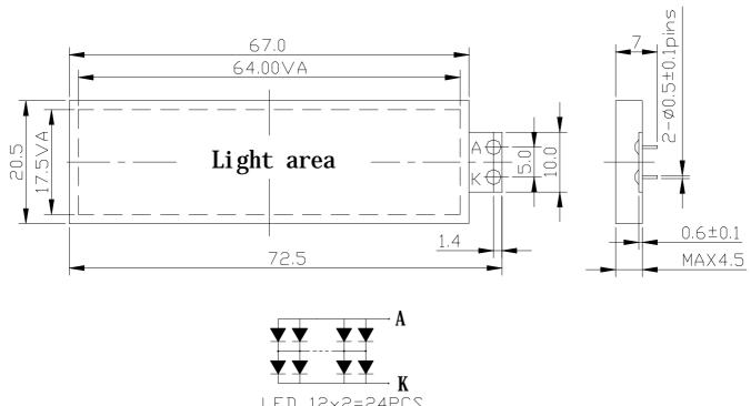
Figure 5.0 LED-Plan for DEM 16216 FGH-LA-N
