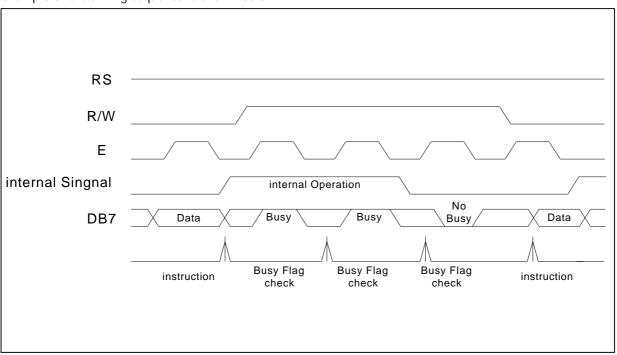
Figure 6.0 Example of 8-bit bus mode timing diagram
