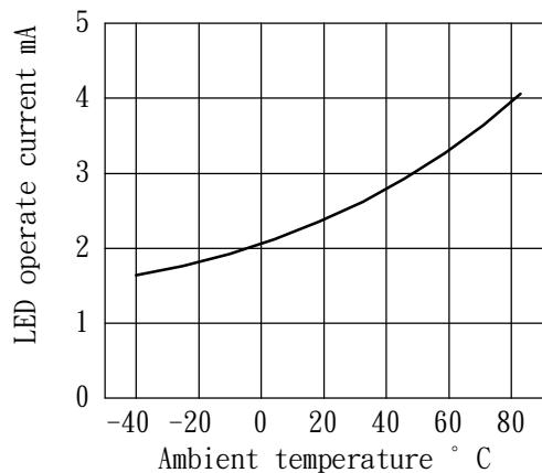
LED turn off current vs. ambient temperature
