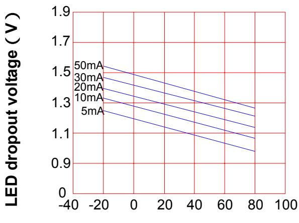
Voltage vs. current characteristics
