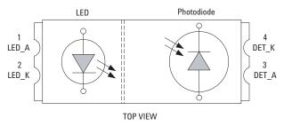
Figure 1. Block Layout of HSDL-9100
