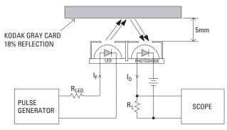
Figure 4. Response Time Test Condition
