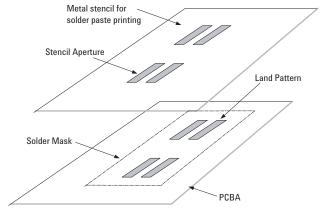
Figure 9. Stencil and PCBA
