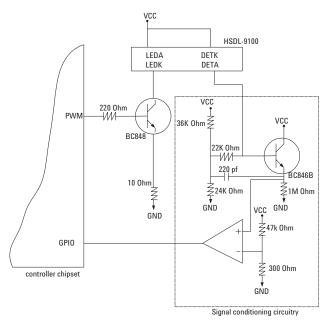
Figure 15. HSDL9100 configuration with controller chipset
