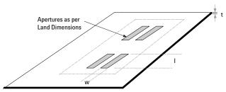
Figure 11. Solder stencil aperture
