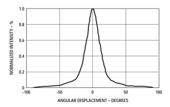
Figure 6. Representative spatial radiation pattern for 23 $^{\circ}$  viewing angle lamps
