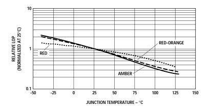
Figure 8. Relative light output vs. junction temperature
