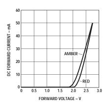
Figure 2a. Forward current vs. forward voltage for option -xxRxx, -xxSxx, -xxTxx, -xxUxx, -xxWxx and -xxYxx
