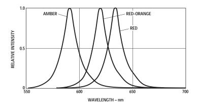
Figure 1. Relative intensity vs. peak wavelength
