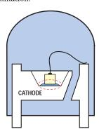
**Note:** Electrical connection between bottom surface of LED die and the lead frame material through conductive paste of solder.
