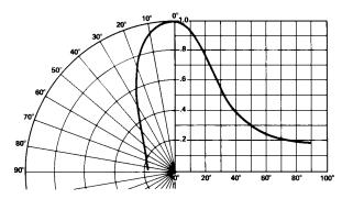
Figure 16. Relative luminous intensity vs. angular displacement.
