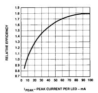
Figure 14. Relative efficiency (luminous intensity per unit vurrent) vs. peak LED current.
