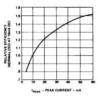
Figure 9. Relative efficiency (luminous intensity per unit current) vs. peak current.
