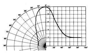
Figure 11. Relative luminous intensity vs. angular displacement.
