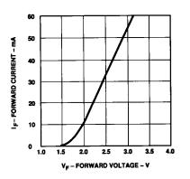
Figure 7. Forward current vs. forward voltage
