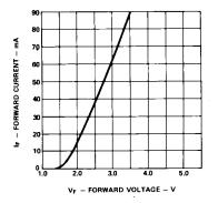
Figure 2. Forward current vs. forward voltage characteristics.
