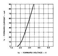
Figure 12. Forward current vs. forward
