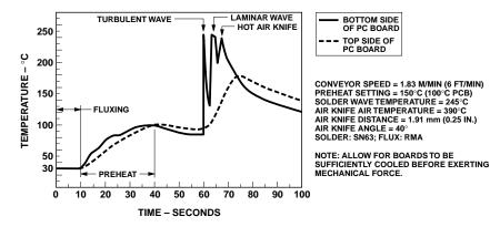
Figure 17. Recommended wave soldering profile.
