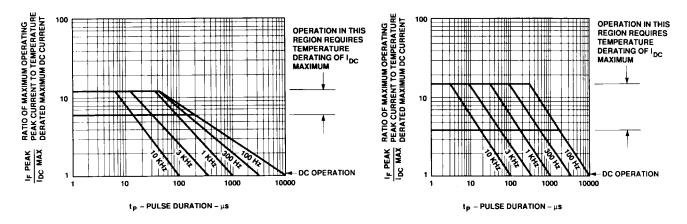
Figure 1. Maximum Tolerable Peak Current vs. **Pulse Duration - Red.**
