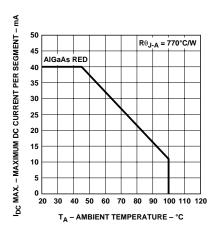
Figure 3. Maximum Allowable DC Current vs. Ambient Temperature.
