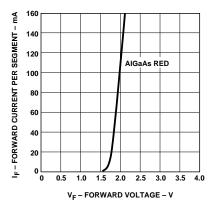
Figure 4. Forward Current vs. Forward Voltage.
