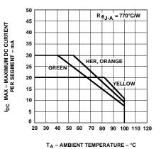
Figure 10. Maximum Allowable DC Current vs. Ambient Temperature.
