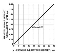
Figure 5. Relative Luminous Intensity vs. DC Forward Current.
