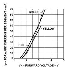
Figure 2. Forward current vs. forward voltage.
