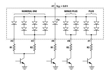
Figure 3. Typical driving circuit.
