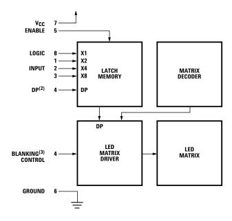
Figure 2. Logic block diagram.
