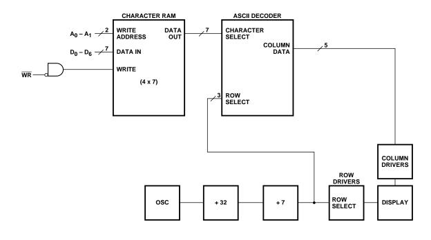
Figure 2. Display internal block diagram.
