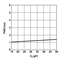
Figure 8. Typical pulse width distortion vs. output load capacitance.
