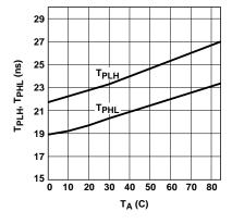
Figure 3. Typical propagation delays vs. temperature.
