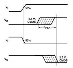
Figure 13. Propagation delay skew waveform.
