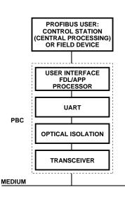
Figure 22. PROFIBUS Controller (PBC).
