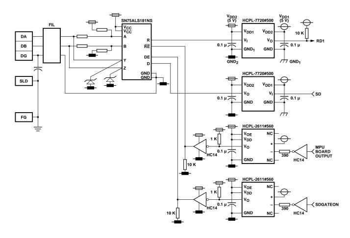
Figure 17. Recommended CC-Link application circuit.
