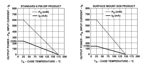
Figure 9. Thermal derating curve, dependence of safety limiting value with case temperature per IEC/EN/DIN EN 60747-5-2.
