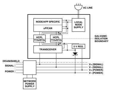
Figure 16. Typical DeviceNet Node.
