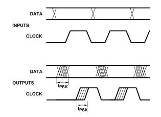
Figure 14. Parallel data transmission example.
