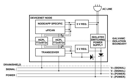
the transceiver and isolated (network) side of the two optocouplers. This method is recommended when there are a limited number of devices on the network that don't require much power, thus eliminating the need for separate power supplies.
