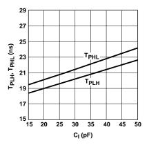
Figure 7. Typical propagation delays vs. output load capacitance.
