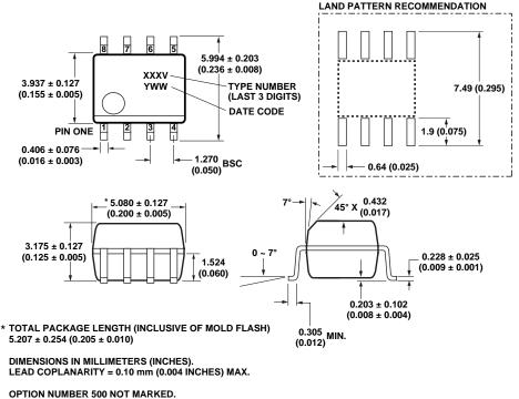
NOTE: FLOATING LEAD PROTRUSION IS 0.15 mm (6 mils) MAX.
