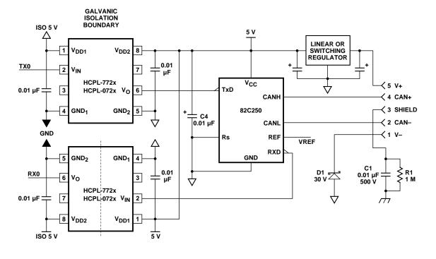
Figure 21. Recommended DeviceNet application circuit.
