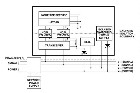
Isolated Node with Transceiver Powered by the Network (Figure 19), and Isolated Node Providing Power to the Network (Figure 20).
