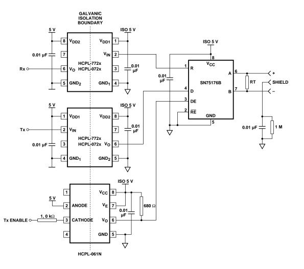
Figure 23. Recommended PROFIBUS application circuit.
