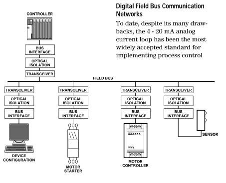
Figure 15. Typical field bus communication physical model.
