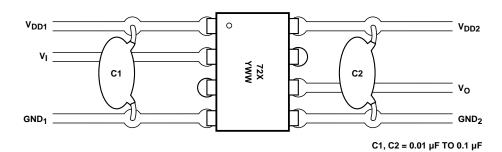
Figure 11. Recommended printed circuit board layout.
