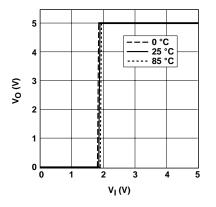
Figure 1. Typical output voltage vs. input voltage.
