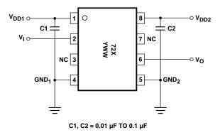
Figure 10. Recommended printed circuit board layout.
