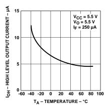
**Figure 1. High Level Output**
