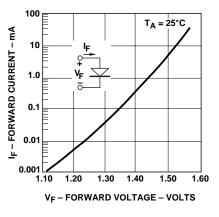
Figure 3. Input Diode Forward Characteristic.
