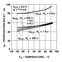
Figure 7. Propagation Delay vs.
