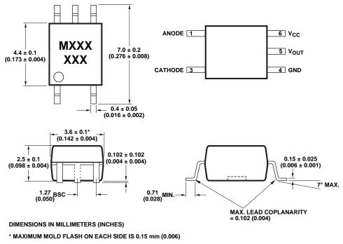
NOTE: FLOATING LEAD PROTRUSION IS 0.15 mm (6 mils) MAX.
