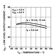
Figure 5. Low Level Output Current vs. Temperature.
