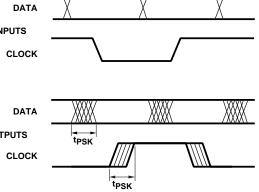
Figure 15. Illustration of Propagation Delay Skew - t<sub>PSK</sub>.
