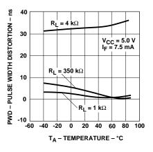
Figure 9. Pulse Width Distortion vs. Temperature.
