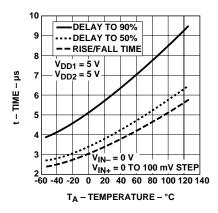
Figure 19. Propagation Delays and Rise/Fall Time vs. Temperature.
