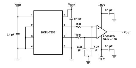
Figure 1. Input Offset Voltage Test Circuit.
