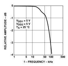
Figure 20. Amplitude Response vs. Frequency.
