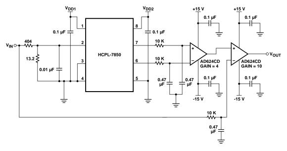
Figure 5. Gain and Nonlinearity Test Circuit.
