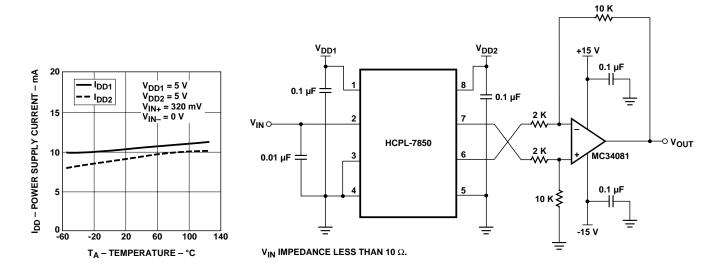
Figure 17. Input and Output Supply Current vs. Temperature.
