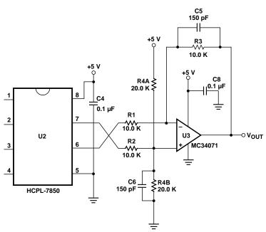
Figure 25. Single-Supply Post-Amplifier Circuit.
