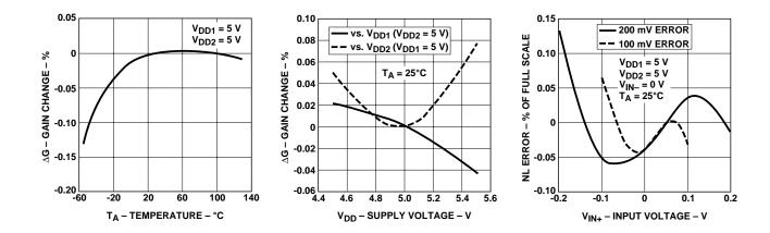
Figure 6. Gain Change vs. Temperature.
