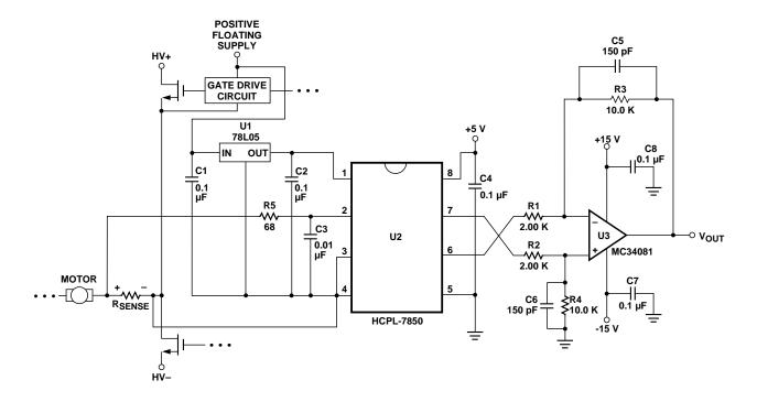
Figure 24. Recommended Application Circuit.
