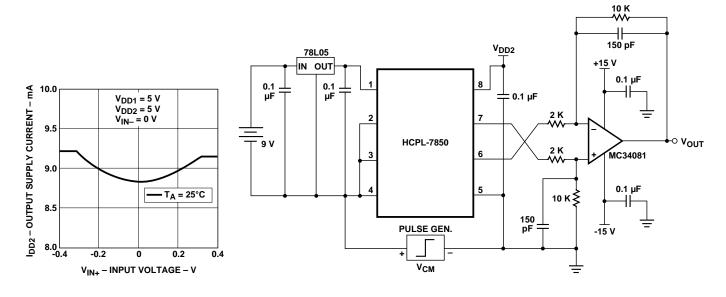
Figure 15. Output Supply Current vs. Input Voltage.
