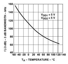
Figure 21. 3 dB Bandwidth vs. Temperature.
