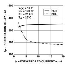
Figure 12. Propagation delay vs. input current
