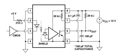
Figure 16. LED drive circuit with resistor connected to LED anode (not recommended)
