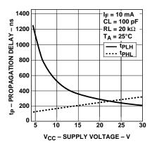
Figure 11. Propagation delay vs. supply voltage
