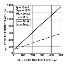
Figure 10. Propagation delay vs. load capacitance
