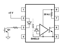
Figure 19. Not recommended open collector LED drive circuit
