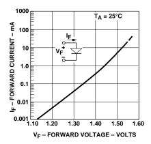
Figure 4. Input current vs. forward voltage
