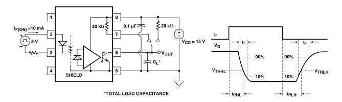
Figure 5. Propagation delay test circuit
