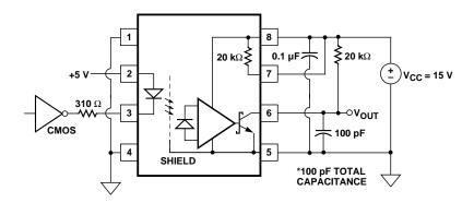
Figure 13. Recommended LED drive circuit
