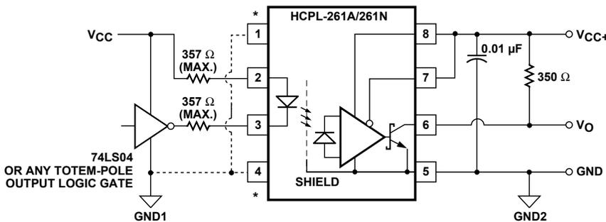
\*Higher CMR may be obtainable by connecting pins 1, 4 to input ground (Gnd1).
