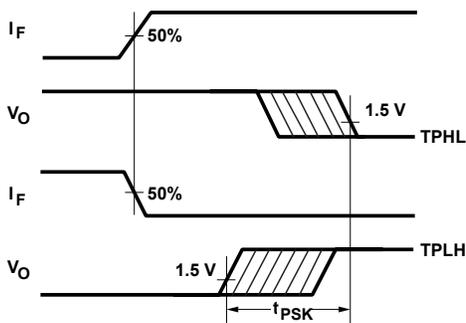
Figure 25. Illustration of propagation delay skew –  $t_{PSK}$ .
