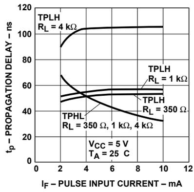
Figure 12. Typical propagation delay vs. pulse input current.
