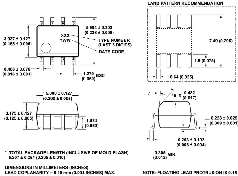
Figure 3. 8-Pin Small Outline Package Device Drawing.
