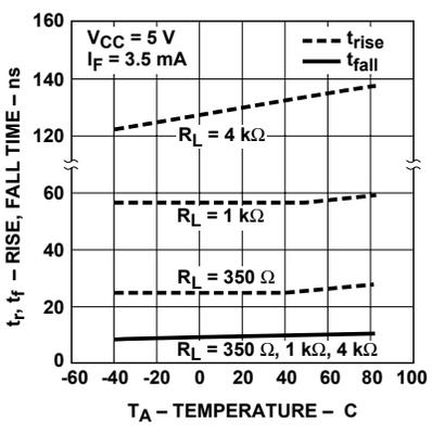
Figure 14. Typical rise and fall time vs. temperature.
