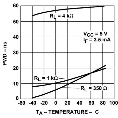
Figure 13. Typical pulse width distortion vs. temperature.
