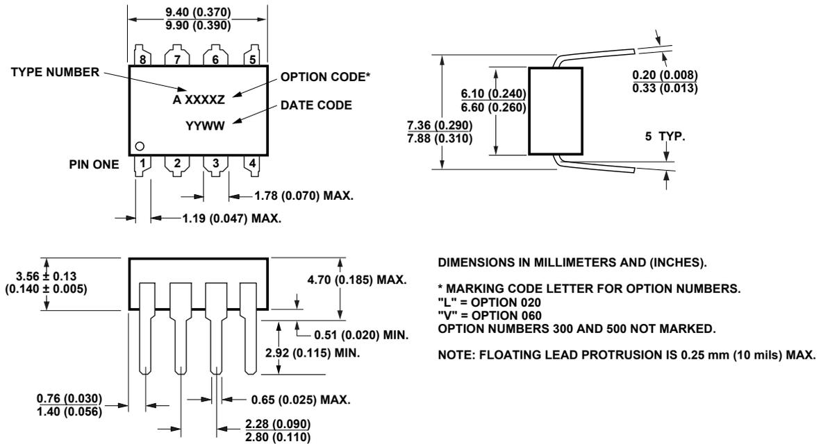
Figure 1. 8-Pin dual in-line package device outline drawing.
