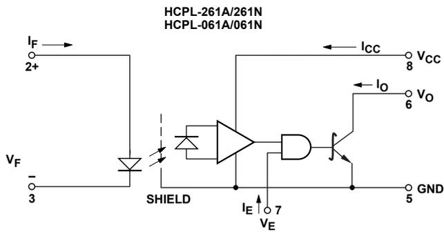
USE OF A 0.1 μF BYPASS CAPACITOR CONNECTED BETWEEN PINS 5 AND 8 IS RECOMMENDED (SEE NOTE 16).
