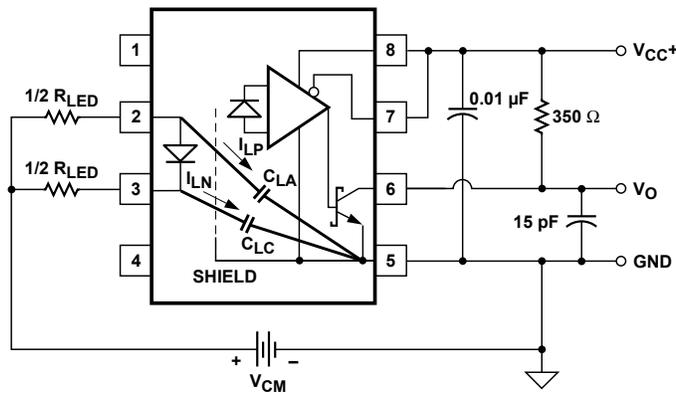
Figure 21. AC equivalent circuit for HCPL-261X.
