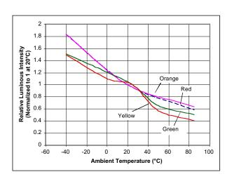
Figure 10. Relative luminous Intensity versus ambient temperature.
