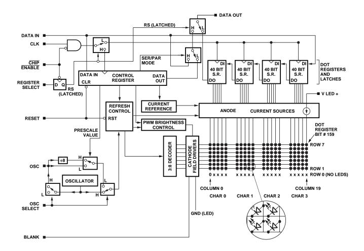
Figure 6. Block diagram for HCMS-39xx.
