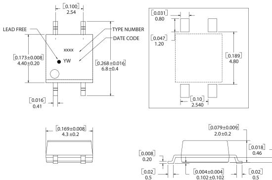
DIMENSIONS IN MILLIMETERS AND [INCHES] OPTION NUMBER 500 AND UL RECOGNITION NOT MARKED
