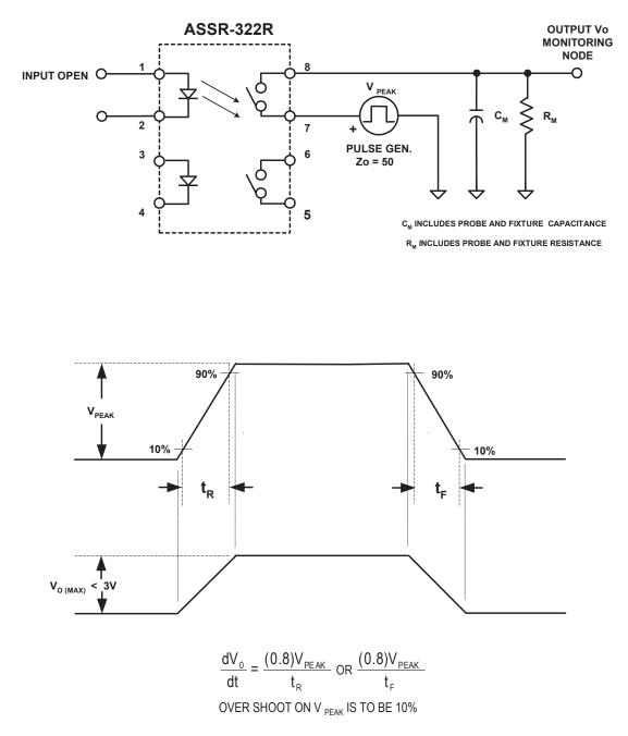
Figure. 15. Output Transient Rejection Test Circuit
