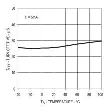
Figure 13. Typical Turn Off Time vs. Temperature
