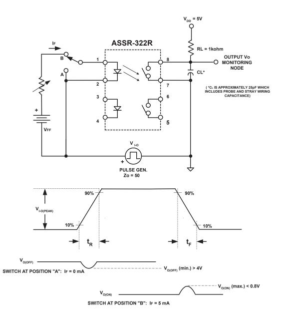
Figure 16. Input-Output Transient Rejection Test Circuit
