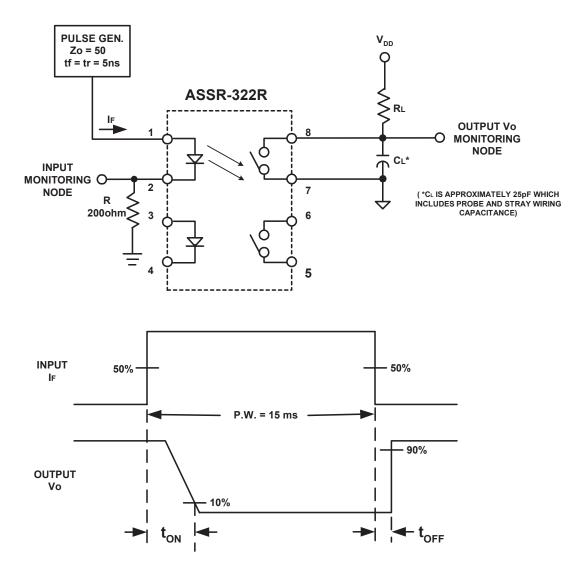
Figure. 14 Switching Test Circuit for TON, TOFF
