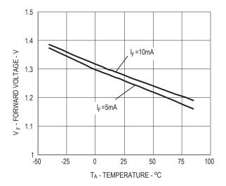
Figure 8. Typical Forward Voltage vs. Temperature
