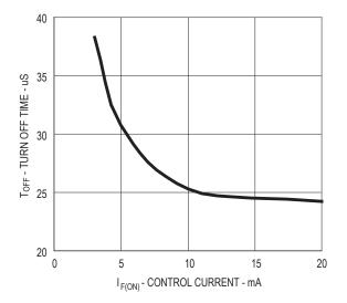
Figure 14. Typical Turn Off Time vs. Input Current
