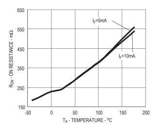
Figure 10. Typical On Resistance vs. Temperature
