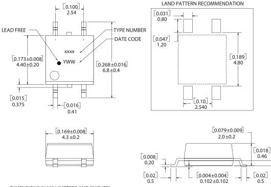
DIMENSIONS IN MILLIMETERS AND [INCHES] OPTION NUMBER 500 AND UL RECOGNITION NOT MARKED
