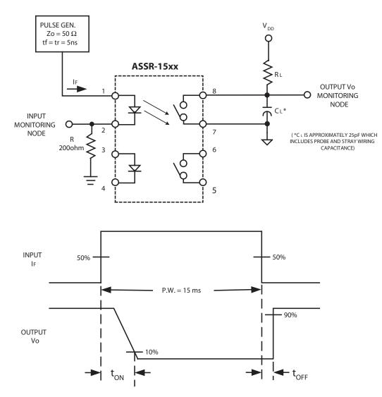
Figure 16. Switching Test circuit for  $t_{\text{ON}}$  ,  $t_{\text{OFF}}$
