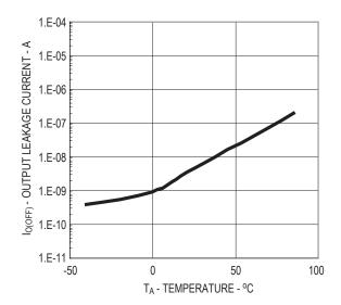
Figure 6. Typical Output Leakage Current vs. Temperature
