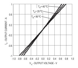
Figure 11. Typical Output Current vs. Output Voltage
