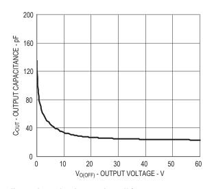
Figure 7. Output Capacitance vs. Output Voltage
