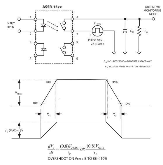
Figure 17. Output Transient Rejection Test Circuit
