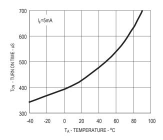
Figure 13. Typical Turn On Time vs. Temperature
