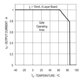
Figure 1. Maximum Output Current Rating vs Ambient Temperature (ASSR-1510-003E)
