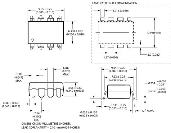
NOTE: FLOATING LEAD PROTRUSION IS 0.25 mm (10 mils) MAX.
