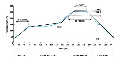
Preheat Temperature 40°C to  $125^{\circ}$ C = 120 sec. max.Temperature Maintain Above  $217^{\circ}$ C = 60 - 150 sec.Peak Temperature=  $255 \pm 5^{\circ}$ CTime Above  $250^{\circ}$ C= 10 - 20 sec.
