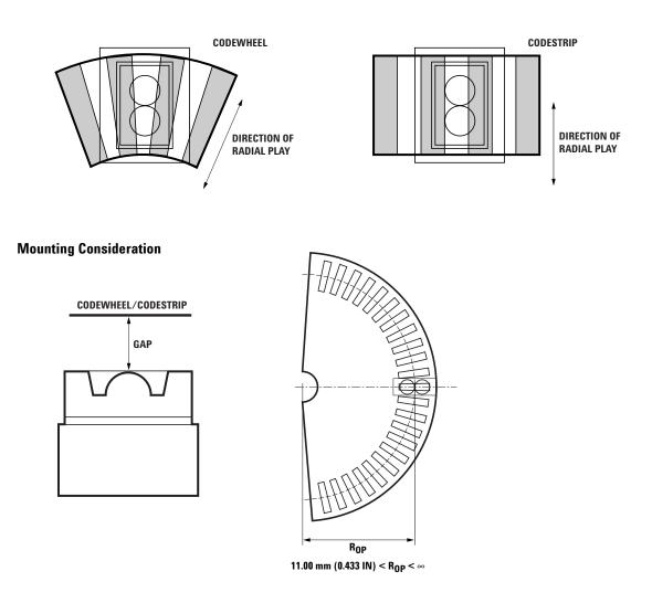
**Direction of Codewheel Rotation** With the emitter side of the encoder placed closer to the codewheel centre, Channel A
