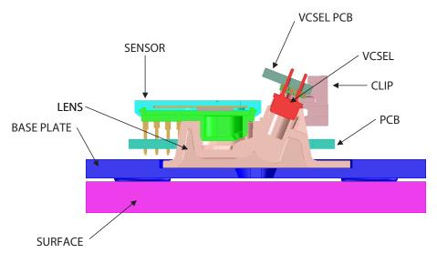
Figure 2. Sectional view of PCB assembly highlighting all optical mouse components (optical mouse sensor, clip, lens, LASER, PCB, and base plate).
