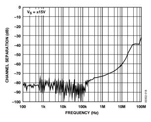
Figure 18. Channel Separation vs. Frequency
