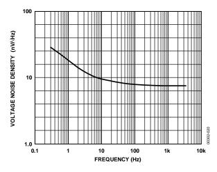
*Figure 20. Voltage Noise Density vs. Frequency*
