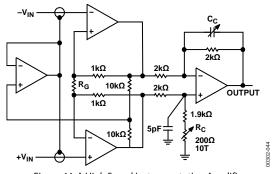
Figure 44. A High Speed Instrumentation Amplifier
