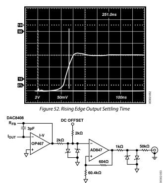
Figure 53. DAC VOUT Settling Time Circuit
