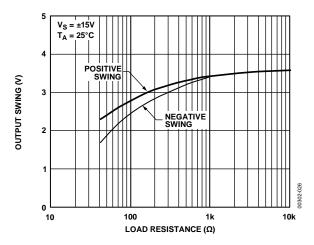
Figure 26. Output Swing vs. Load Resistance
