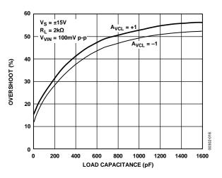
Figure 16. Small Signal Overshoot vs. Load Capacitance
