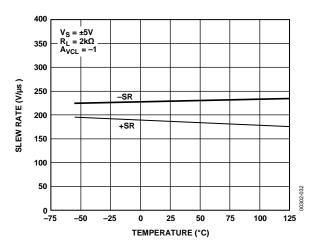
Figure 32. Slew Rate vs. Temperature
