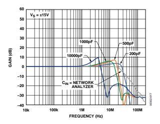
Figure 17. Noninverting Gain vs. Capacitive Loads
