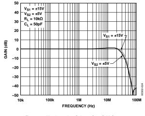
Figure 24. Noninverting Gain vs. Supply Voltage
