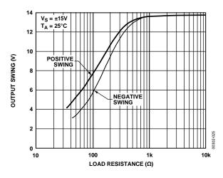
Figure 25. Output Swing vs. Load Resistance
