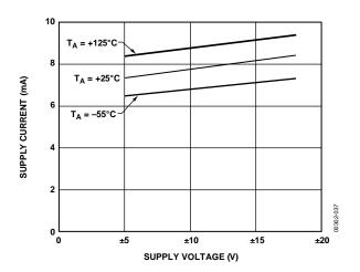
Figure 37. Supply Current vs. Supply Voltage
