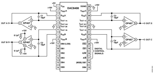
Figure 50. Quad DAC Unipolar Operation
