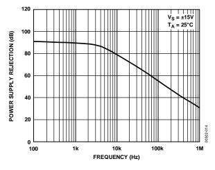
Figure 14. Power-Supply Rejection vs. Frequency
