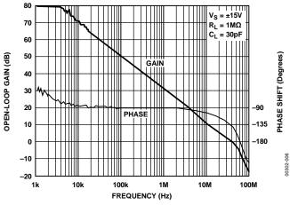
Figure 6. Open-Loop Gain, Phase vs. Frequency
