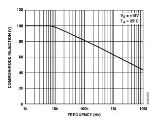
Figure 13. Common-Mode Rejection vs. Frequency
