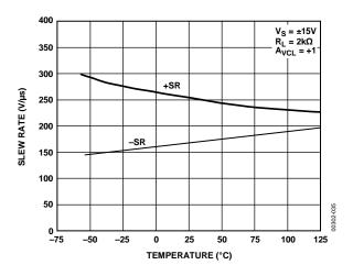
Figure 35. Slew Rate vs. Temperature
