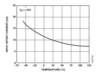
Figure 39. Input Offset Current vs. Temperature
