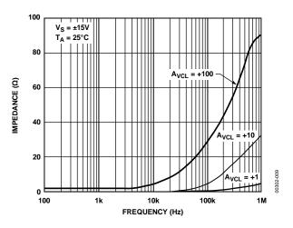
Figure 9. Closed-Loop Output Impedance vs. Frequency
