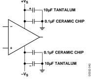
Figure 40. Recommended Power Supply Bypass
