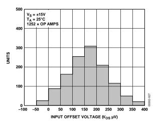
Figure 27. Input Offset Voltage Distribution
