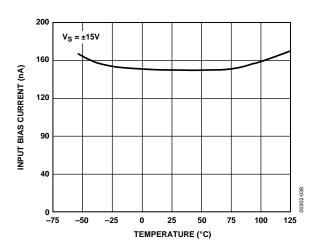
Figure 38. Input Bias Current vs. Temperature
