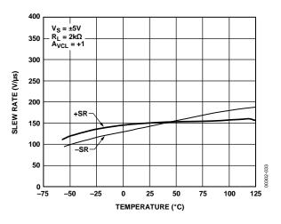
Figure 33. Slew Rate vs. Temperature
