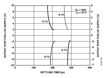
Figure 36. Output Step vs. Settling Time
