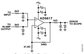
Figure 47. Settling Time Measurement Circuit
