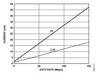
Figure 12. Typical ADuM3440  $V_{DD2}$  Supply Current vs. Data Rate for 5 V and 3.3 V Operation
