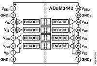
Figure 3. ADuM3442 Functional Block Diagram
