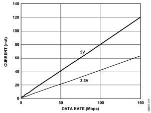
Figure 11. Typical ADuM3440 V<sub>DD1</sub> Supply Current vs. Data Rate for 5 V and 3.3 V Operation
