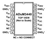
\*PIN 2 AND PIN 8 ARE INTERNALLY CONNECTED AND CONNECTING BOTH TO  $\mathrm{GND}_1$  IS RECOMMENDED. PIN 9 AND PIN 15 ARE INTERNALLY CONNECTED AND CONNECTING BOTH TO  $\mathrm{GND}_2$  IS RECOMMENDED.
