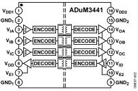
Figure 2. ADuM3441 Functional Block Diagram
