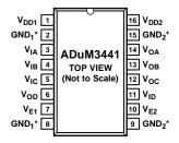
\*PIN 2 AND PIN 8 ARE INTERNALLY CONNECTED AND CONNECTING BOTH TO  ${\rm GND_1}$  IS RECOMMENDED. PIN 9 AND PIN 15 ARE INTERNALLY CONNECTED AND CONNECTING BOTH TO  ${\rm GND_2}$  IS RECOMMENDED.
