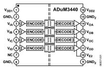
Figure 1. ADuM3440 Functional Block Diagram
