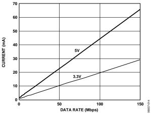
Figure 14. Typical ADuM3441  $V_{\rm DD2}$  Supply Current vs. Data Rate for 5 V and 3.3 V Operation
