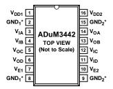
\*PIN 2 AND PIN 8 ARE INTERNALLY CONNECTED AND CONNECTING BOTH TO  ${\rm GND_1}$  IS RECOMMENDED. PIN 9 AND PIN 15 ARE INTERNALLY CONNECTED AND CONNECTING BOTH TO  ${\rm GND_2}$  IS RECOMMENDED.
