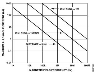
Figure 19. Maximum Allowable Current for Various Current-to-ADuM344x Spacings
