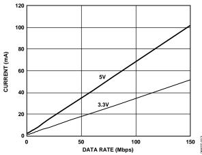
Figure 13. Typical ADuM3441 V<sub>DD1</sub> Supply Current vs. Data Rate for 5 V and 3.3 V Operation
