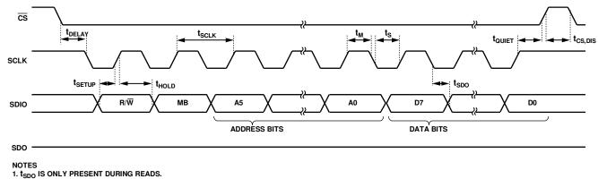
Figure 31. SPI 3-Wire Read/Write
