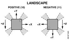
Figure 42. 2-D Orientation with Corresponding Codes
