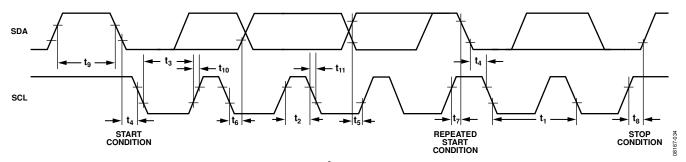
Figure 34. I<sup>2</sup>C Timing Diagram
