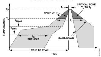
Figure 47. Recommended Soldering Profile
