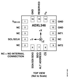
Figure 2. Pin Configuration (Top View)
