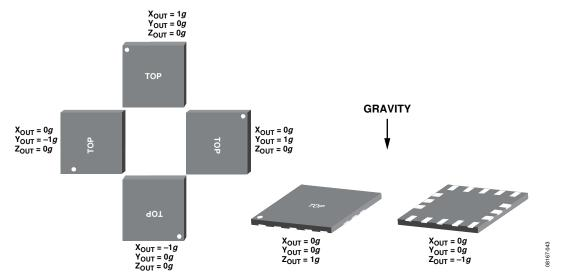
Figure 45. Output Response vs. Orientation to Gravity
