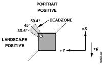
Figure 43. Orientation Showing a 10.8° Dead Zone Region
