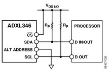
Figure 32. I<sup>2</sup>C Connection Diagram (Address 0x53)
