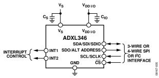
Figure 36. Application Diagram
