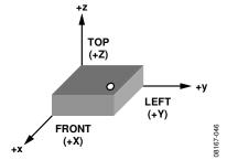
Figure 41. 3-D Orientation with Coordinate System
