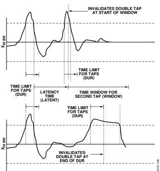
Figure 40. Tap Interrupt Function with Invalid Double Taps
