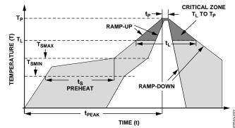
Figure 3. Soldering Profile Diagram
