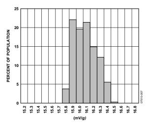
Figure 7. Sensitivity Distribution (3.3 V Supply, 25°C)
