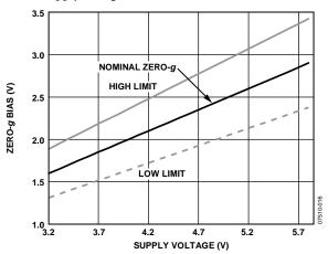
Figure 16. Typical Zero-q Bias Levels Across Varying Supply Voltages
