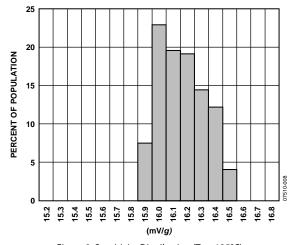
Figure 8. Sensitivity Distribution ( $T_A = 125$ °C)
