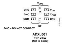
Figure 4. Pin Configuration
