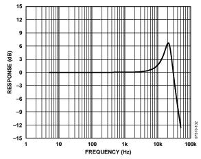
Figure 1. Sensor Frequency Response
