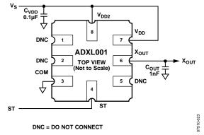
Figure 14. Application Circuit
