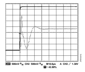
Figure 12. Turn-On Characteristic (10 µs per DIV)
