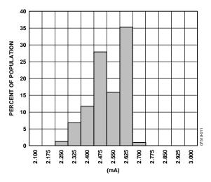
Figure 11.  $I_{SUPPLY}$  at 125°C
