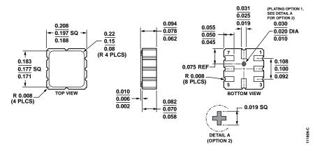
Figure 17. 8-Terminal Ceramic Leadless Chip Carrier [LCC] (E-8-1) Dimensions shown in inches
