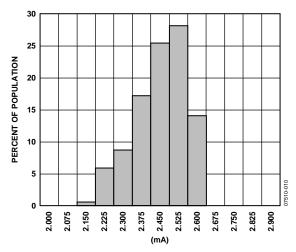
Figure 10. Isupply at 25°C
