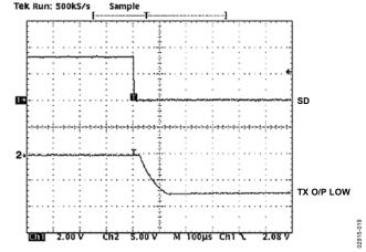
Figure 19. Transmitter Output (Low) Exiting Shutdown
