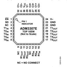
Figure 4. ADM3307E LFCSP\_VQ Pin Configuration
