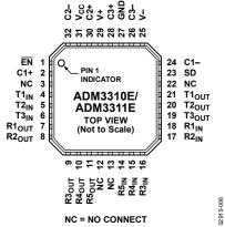
Figure 6. LFCSP\_VQ Pin Configuration
