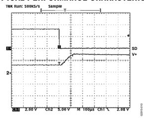
Figure 10. Charge Pump V+ Exiting Shutdown
