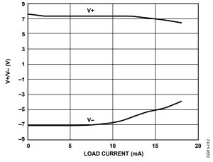
Figure 12. Charge Pump V+/V- vs. Load Current (V<sub>CC</sub> = 3.3 V)
