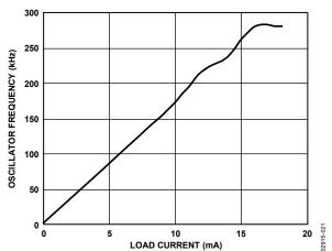
Figure 21. Oscillator Frequency vs. Load Current
