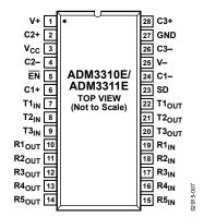
Figure 7. SSOP/TSSOP Pin Configuration
