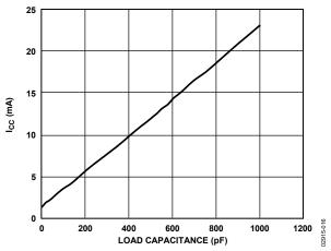
Figure 16. Supply Current vs. Load Capacitance ( $R_L$  = Infinite) ( $V_{CC}$  = 3.3 V, Data Rate = 460 kbps)
