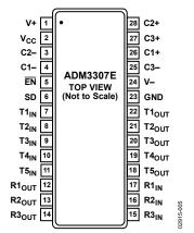
Figure 5. SSOP/TSSOP Pin Configuration
