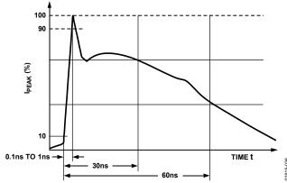
Figure 36. IEC1000-4-2 ESD Current Waveform
