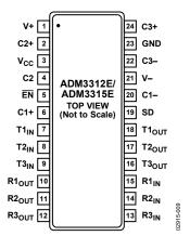
Figure 9. SSOP/TSSOP Pin Configuration
