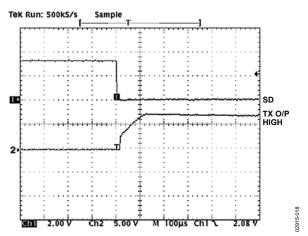
Figure 18. Transmitter Output (High) Exiting Shutdown
