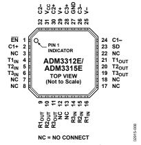
Figure 8. LFCSP\_VQ Pin Configuration
