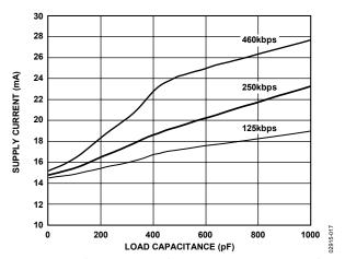
Figure 17. Supply Current vs. Load Capacitance ( $V_{CC} = 3.3 V$ ,  $R_L = 5 k\Omega$ )
