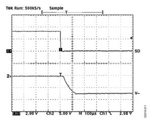
Figure 11. Charge Pump V – Exiting Shutdown
