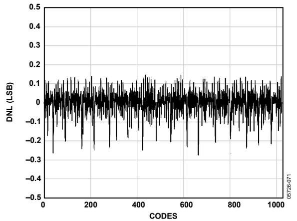
Figure 38. DNL,  $f_{IN} = 2.4$  MHz,  $f_{SAMPLE} = 65$  MSPS
