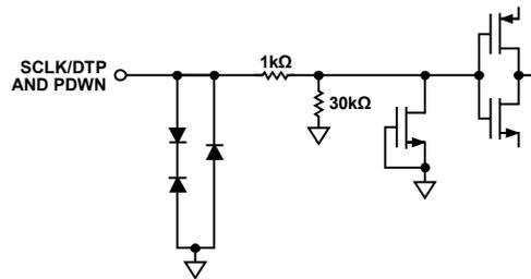
Figure 10. Equivalent SCLK/DTP and PDWN Input Circuit
