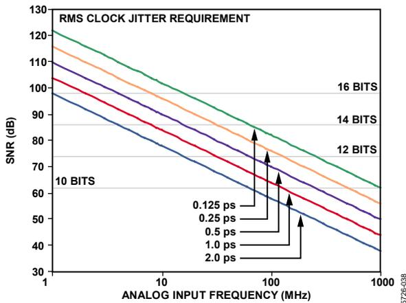
Figure 57. Ideal SNR vs. Input Frequency and Jitter
