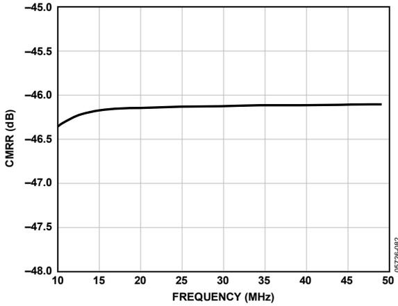
Figure 39. CMRR vs. Frequency,  $f_{SAMPLE} = 65$  MSPS
