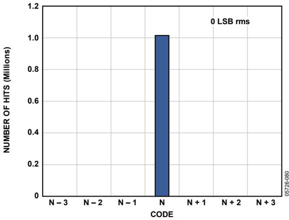
Figure 40. Input-Referred Noise Histogram,  $f_{SAMPLE} = 65$  MSPS
