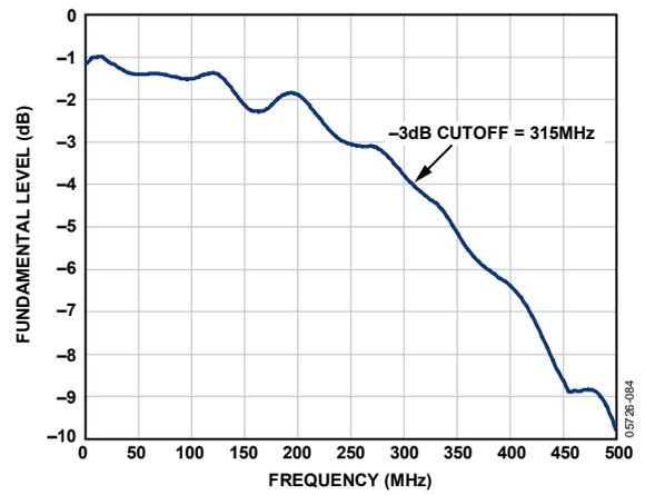
Figure 42. Full-Power Bandwidth vs. Frequency,  $f_{SAMPLE} = 65$  MSPS
