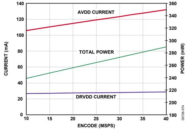
Figure 58. Supply Current vs.  $f_{SAMPLE}$  for  $f_{IN} = 10.3 \text{ MHz}$ ,  $f_{SAMPLE} = 40 \text{ MSPS}$
