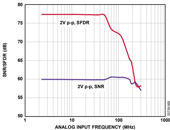
Figure 35. SNR/SFDR vs. Analog Input Frequency,  $f_{SAMPLE} = 65$  MSPS
