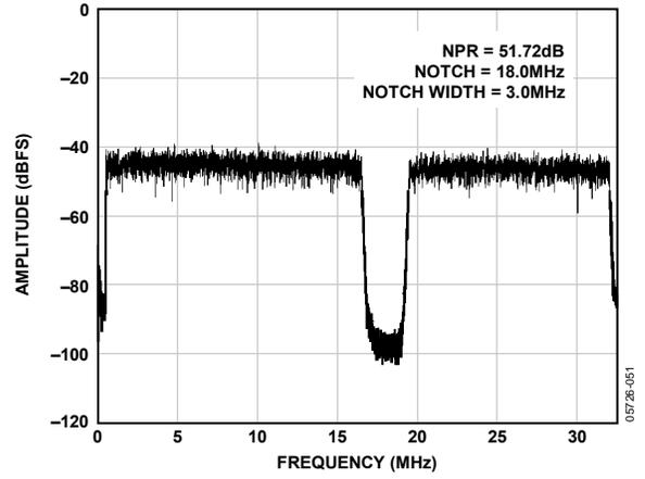
Figure 41. Noise Power Ratio (NPR),  $f_{SAMPLE} = 65$  MSPS
