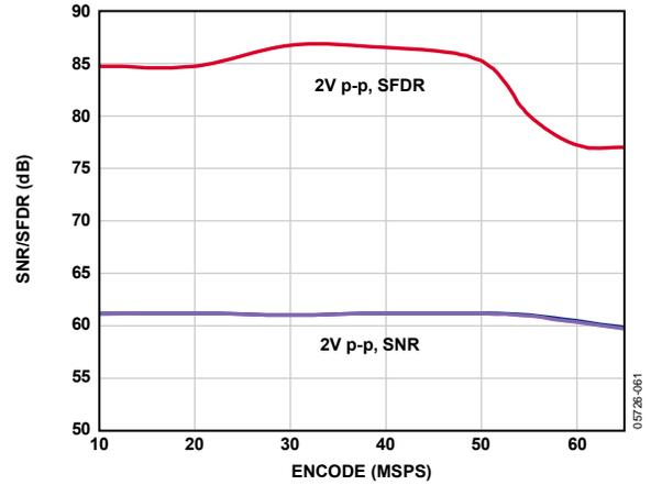
Figure 25. SNR/SFDR vs. Encode,  $f_{IN} = 10.3$  MHz,  $f_{SAMPLE} = 65$  MSPS
