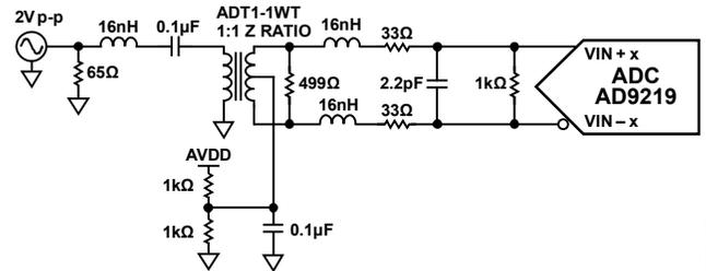
Figure 49. Differential Transformer-Coupled Configuration for IF Applications
