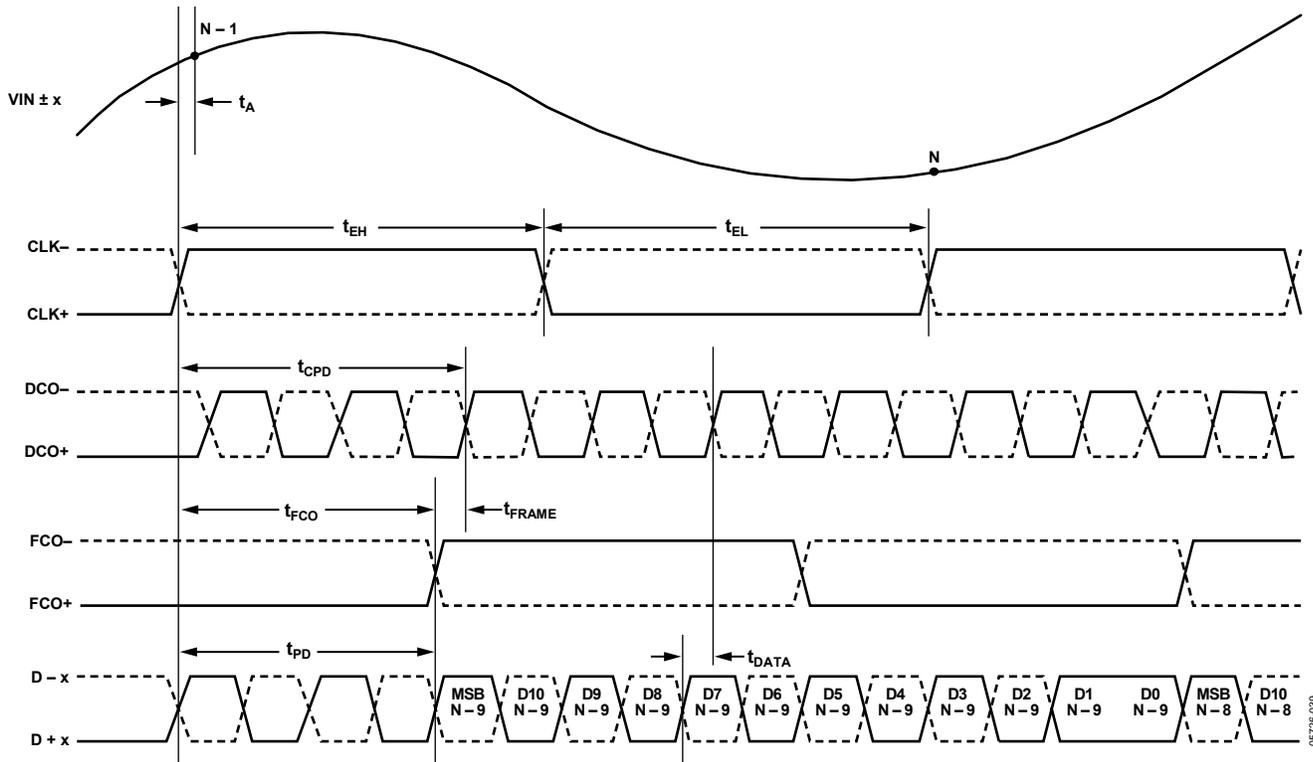
Figure 3. 12-Bit Data Serial Stream, MSB First
