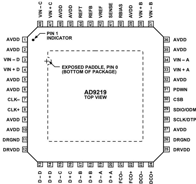
Figure 5. 48-Lead LFCSP Pin Configuration, Top View
