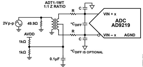
Figure 48. Differential Transformer-Coupled Configuration for Baseband Applications
