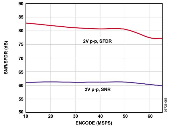
Figure 26. SNR/SFDR vs. Encode,  $f_{IN} = 35$  MHz,  $f_{SAMPLE} = 65$  MSPS
