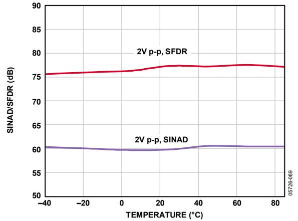
Figure 36. SINAD/SFDR vs. Temperature,  $f_{IN} = 10.3$  MHz,  $f_{SAMPLE} = 65$  MSPS
