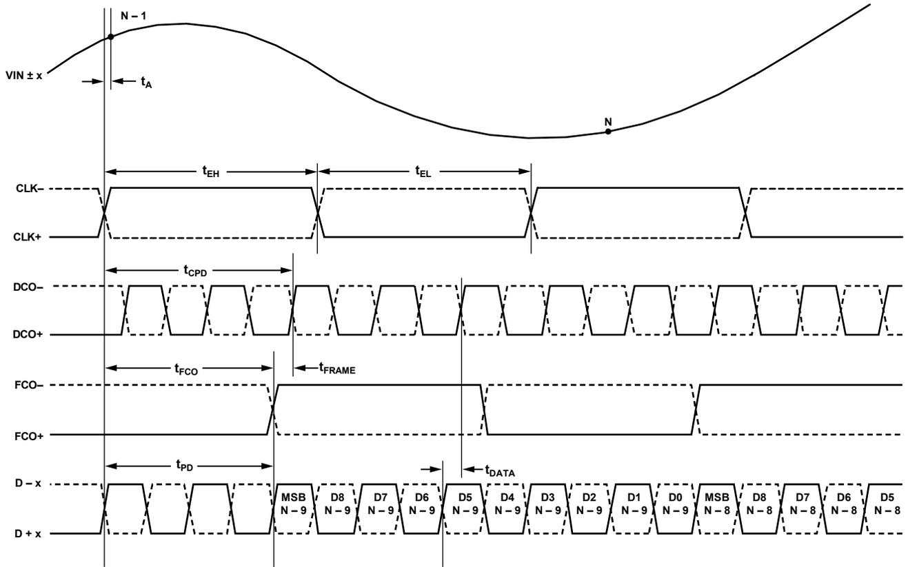
Figure 2. 10-Bit Data Serial Stream, MSB First (Default)
