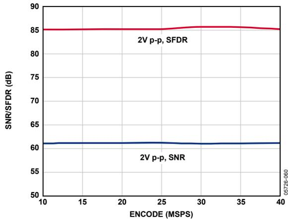
Figure 23. SNR/SFDR vs. Encode,  $f_{IN} = 10.3$  MHz,  $f_{SAMPLE} = 40$  MSPS
