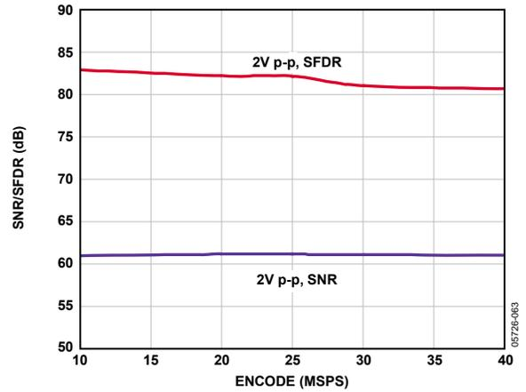
Figure 24. SNR/SFDR vs. Encode,  $f_{IN} = 35$  MHz,  $f_{SAMPLE} = 40$  MSPS
