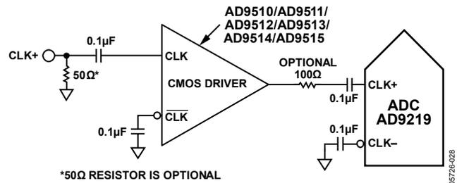
Figure 56. Single-Ended 3.3 V CMOS Sample Clock
