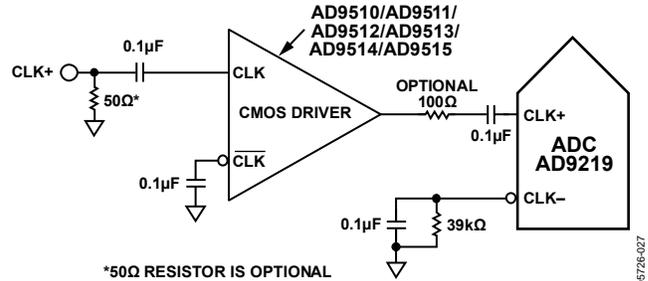
Figure 55. Single-Ended 1.8 V CMOS Sample Clock
