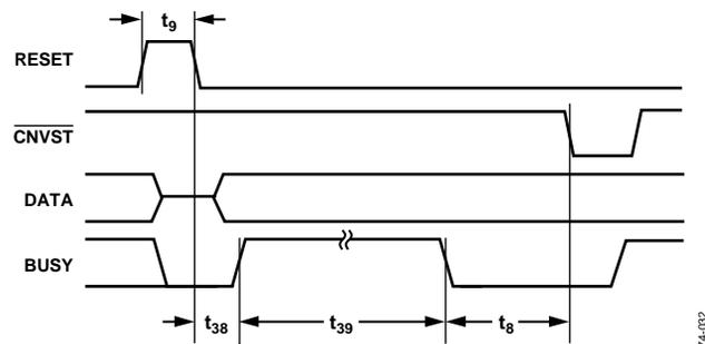
Figure 32. RESET Timing
