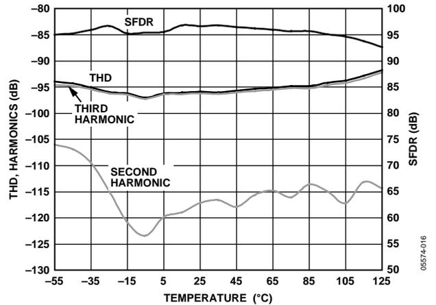
Figure 16. THD, Harmonics, and SFDR vs. Temperature
