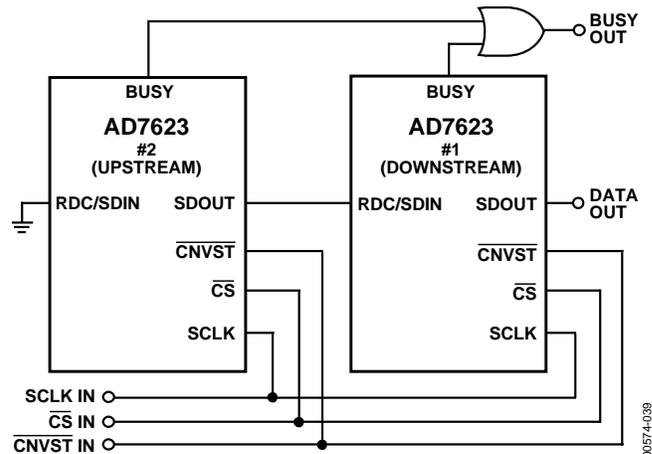
Figure 39. Two AD7623 Devices in a Daisy-Chain Configuration
