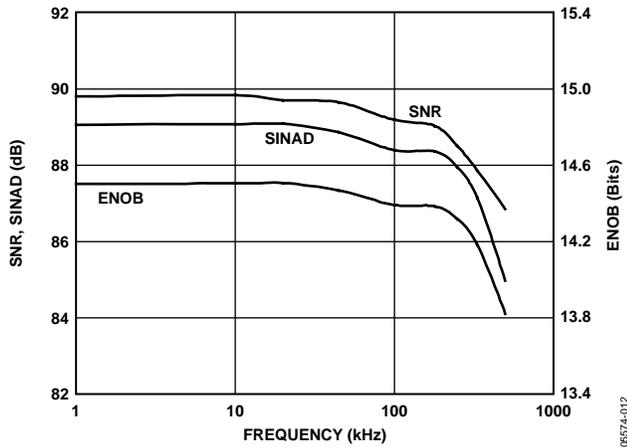
Figure 12. SNR, SINAD and ENOB vs. Frequency
