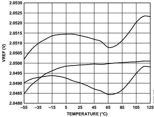
Figure 7. Typical Reference Voltage Output vs. Temperature (3 Units)
