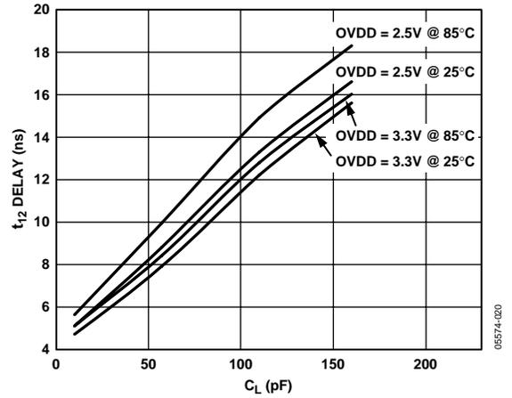
Figure 20. Typical Delay vs. Load Capacitance  $C_L$
