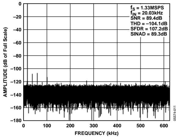
Figure 11. FFT 20 kHz
