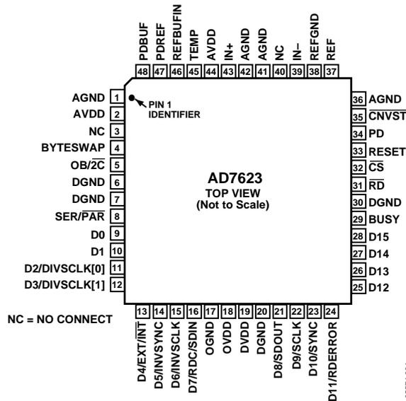
Figure 4. Pin Configuration
