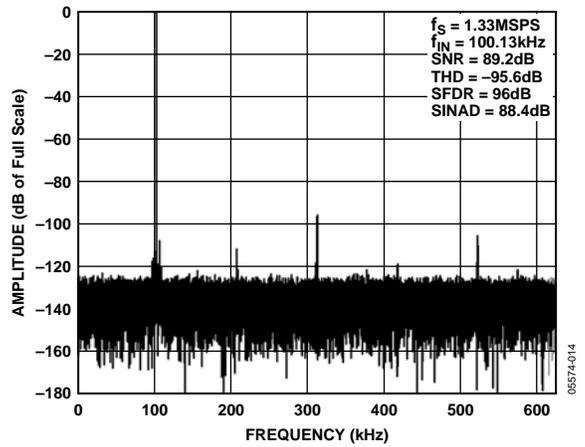
Figure 14. FFT 100 kHz
