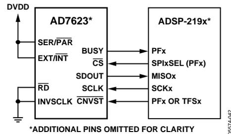
Figure 42. Interfacing the AD7623 to SPI Interface
