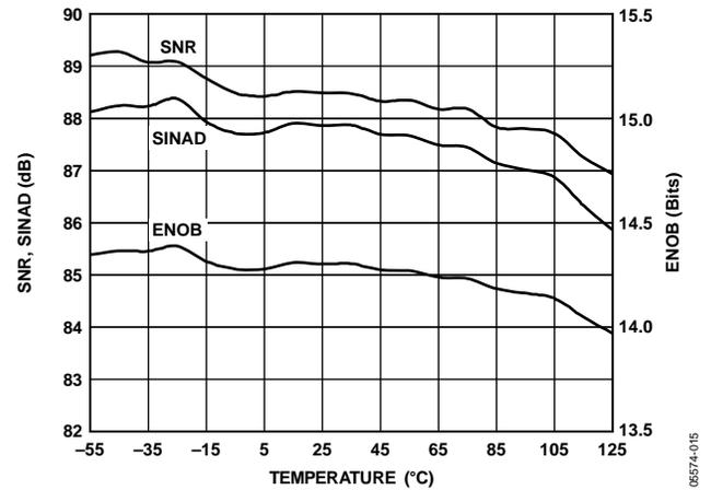
Figure 15. SNR, SINAD, and ENOB vs. Temperature
